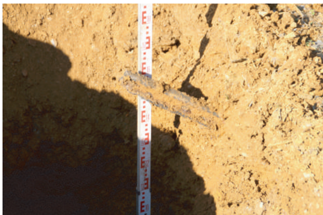
Plate 19. Detail shot showing remains of tram rail protruding through spoil close to Adit No.9. in Trial Pit No. 7. Looking westwards.
