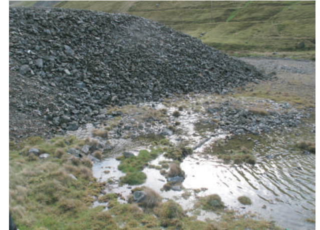
Plate 18. Leachig of water from spoil tip alongside Gill's Lower Adit. Looking southwest.
