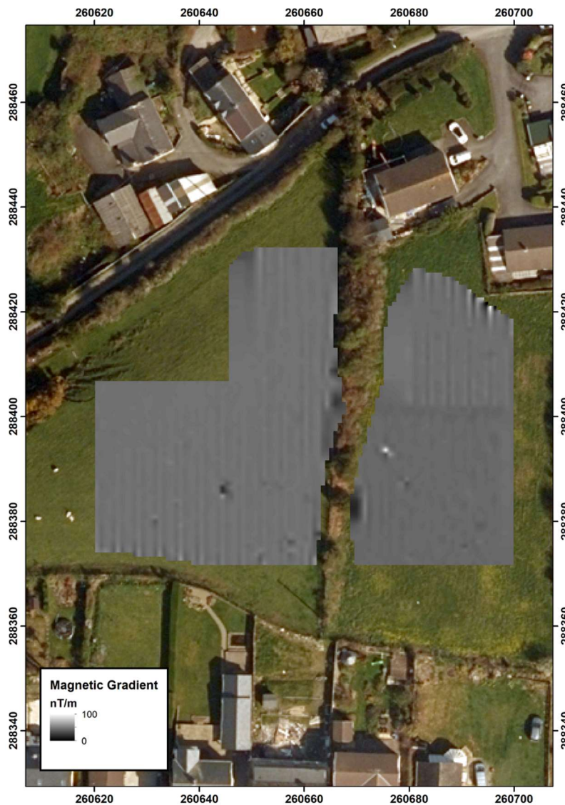
Figure 3. Magnetic Gradient survey data.
