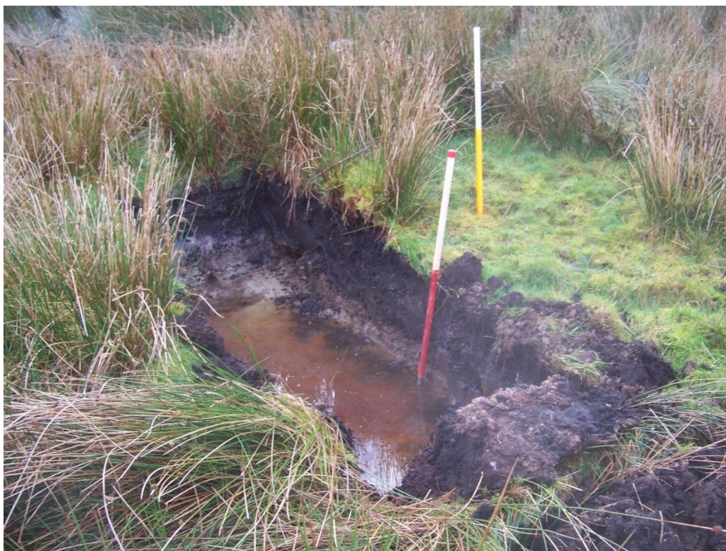
Figure 16 West Inner anchor pit. The peaty topsoil around 0.10m deep is clearly visible as is the yellowy grey clay soil beneath that
