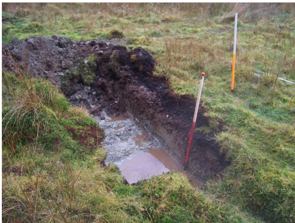
Figure 8 North Inner anchor Pit. The peaty topsoil around 0.10m deep is clearly visible as is the yellowy grey clay beneath that and the shale 0.30m below the surface
