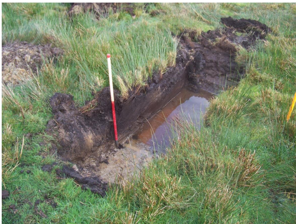
Figure 10 East outer anchor pit. The peaty topsoil up to 0.50m deep is clearly visible as is the yellow grey clay below that
