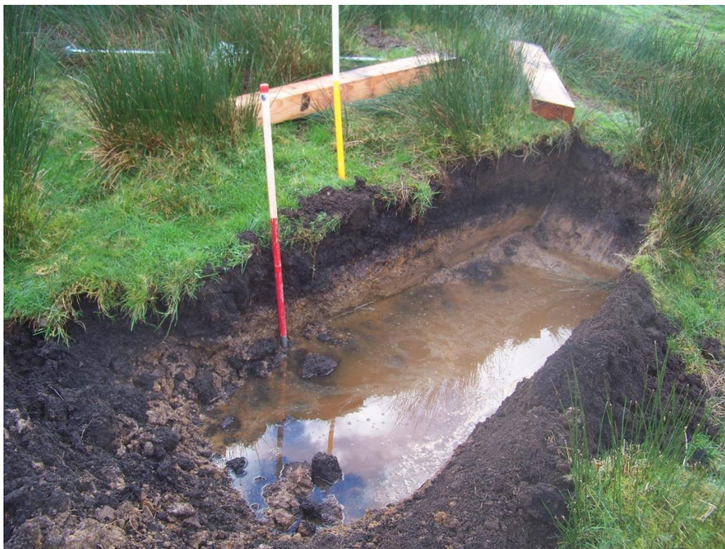
Figure 9 East Inner anchor pit. The peaty topsoil around 0.10m deep is clearly visible as is the yellowy grey clay below that
