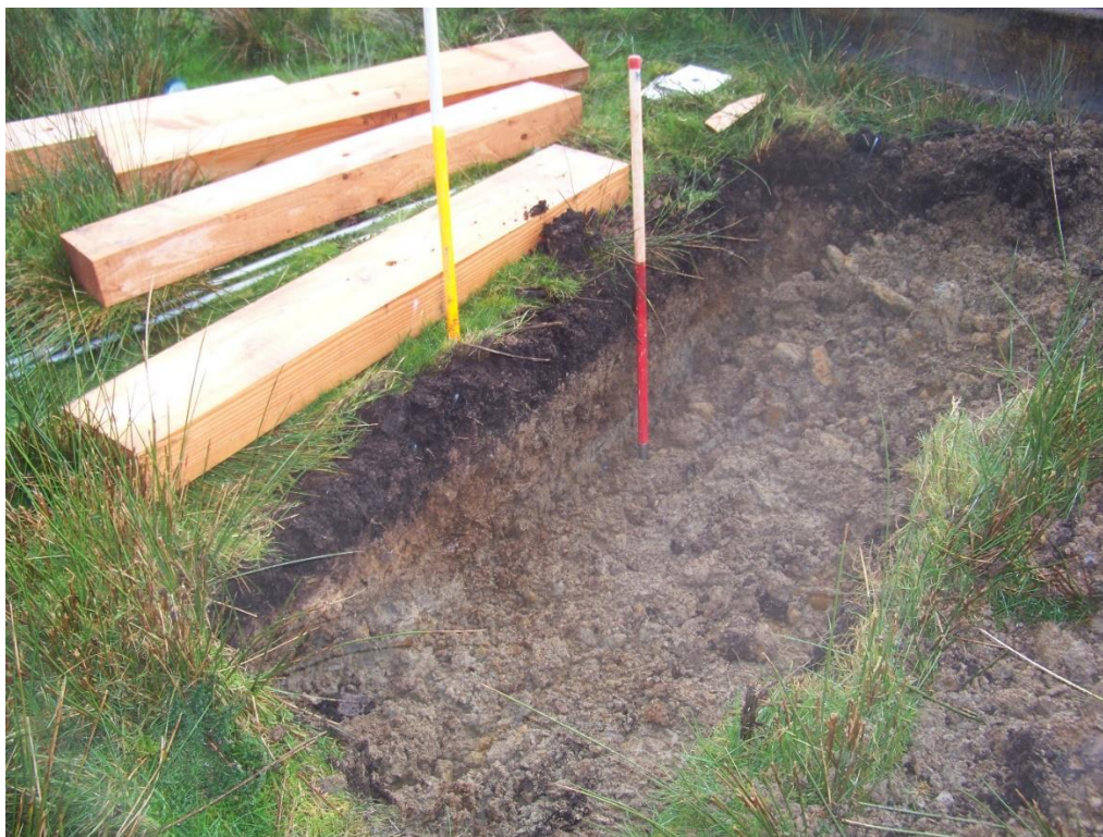
Figure 11 Main Mast Pit. The peaty topsoil around 0.10m deep is clearly visible as is the yellowy grey clay beneath that
