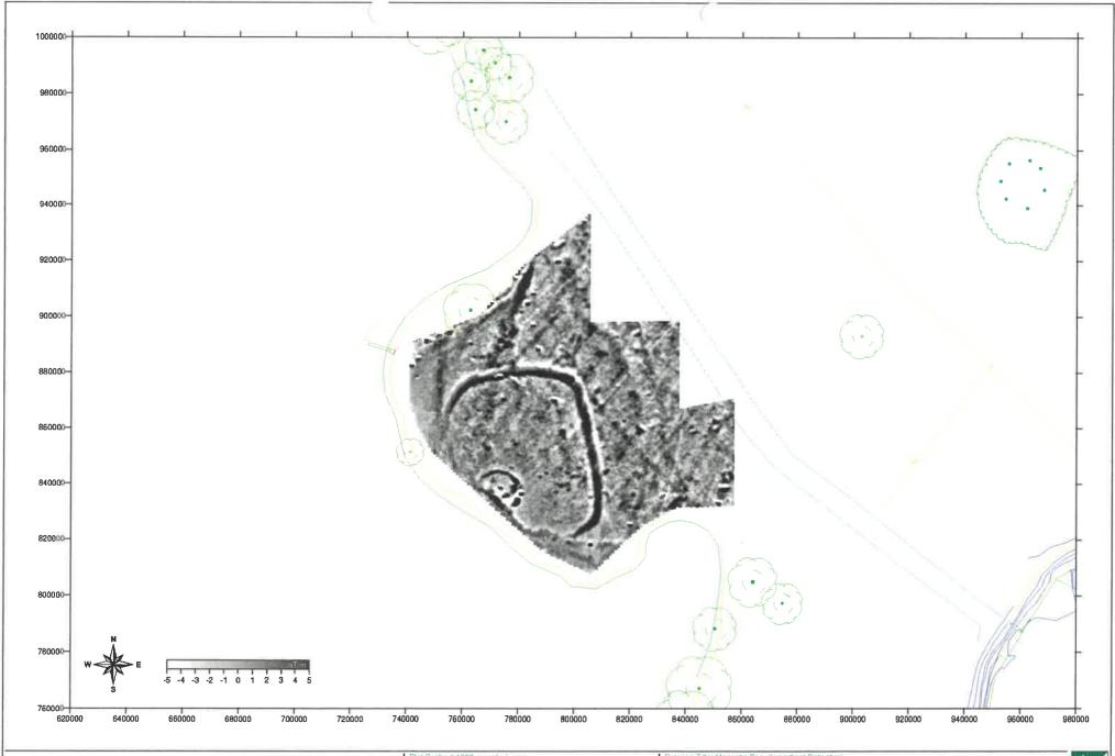
Project Name: Llanerchaeron Enclosure Site Project Code: LLC20041 Plot Scale: 1:1000, coords, in mm Data Resolution: 0.5m x 0.25m Image Resolution: 0.25m x 0.25m Base Mapping: Quintdraft survey, 2000 Drawing Title: Magnetic Pseudogradient Data (1m) = Author: ACKR Version: 1 PRN:
