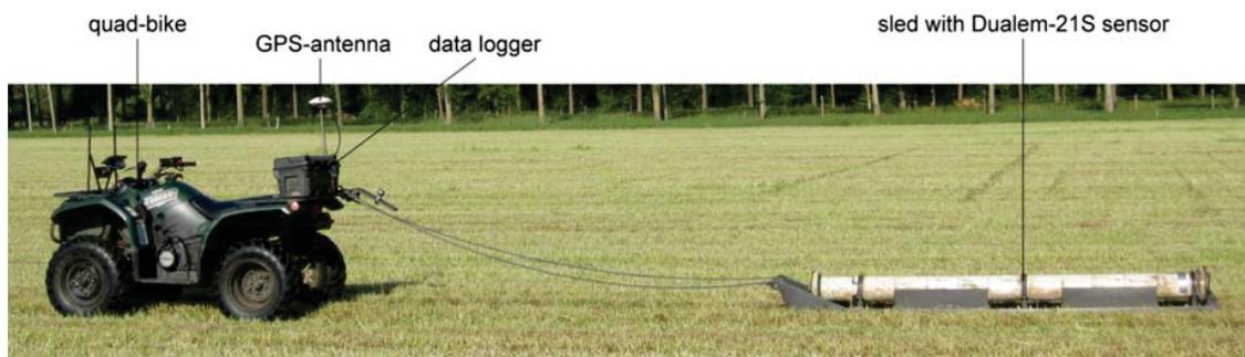
*Fig. 2: Mobile survey configuration with the sled-mounted Dualem-21HS towed by quad-bike with data logger and GPS antenna (From De Smedt et al. (2013a))*
