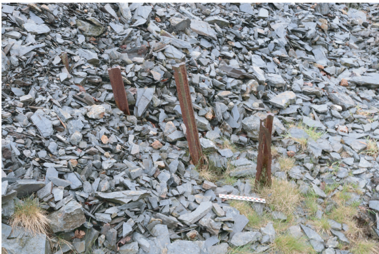
Plate 26. Remains of corroded former iron tramway rails sticking up out of ground in area of proposed new flow gauge at base of spoil tip on east side of stream. May have been used as a temporary fencing at some time across stream bed.
