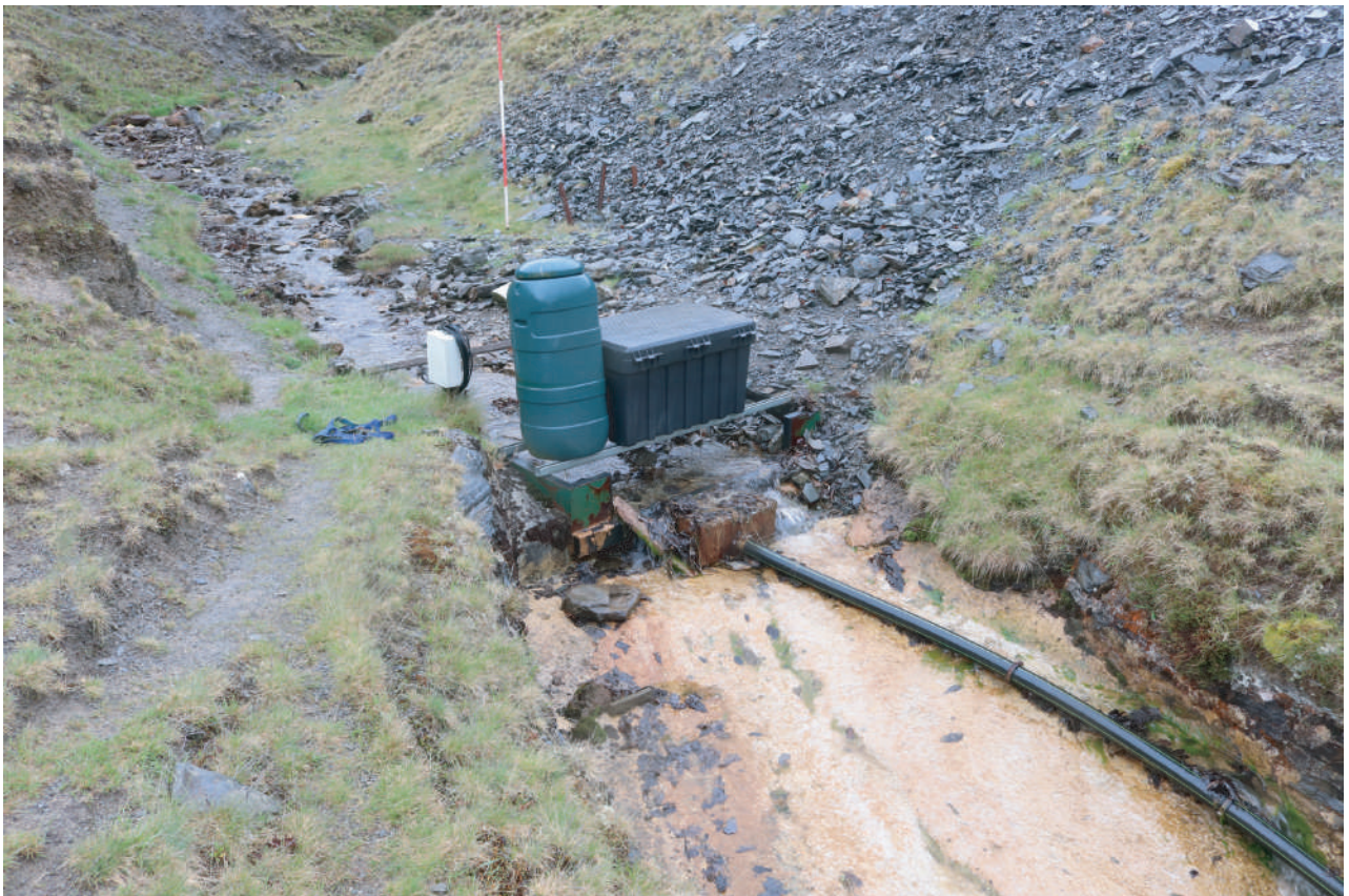
Plate 03. View of existing water flow gauge at discharge point between mine spoil tips. Looking northward.
