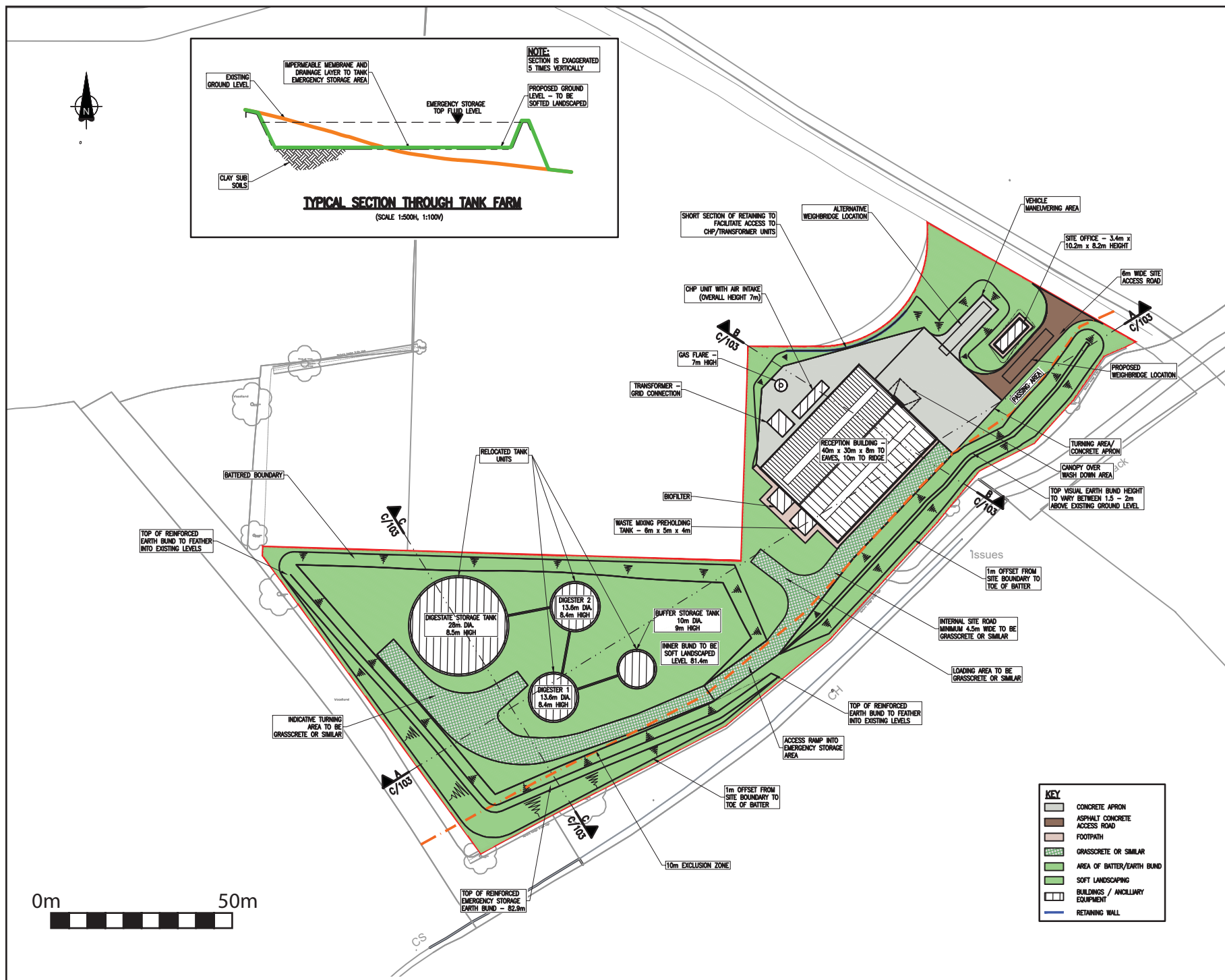
Figure 3: Development plan. Plan produced by Burroughs, drawing No. P/101. Date 27/01/14. Not reproduced to original scale.
