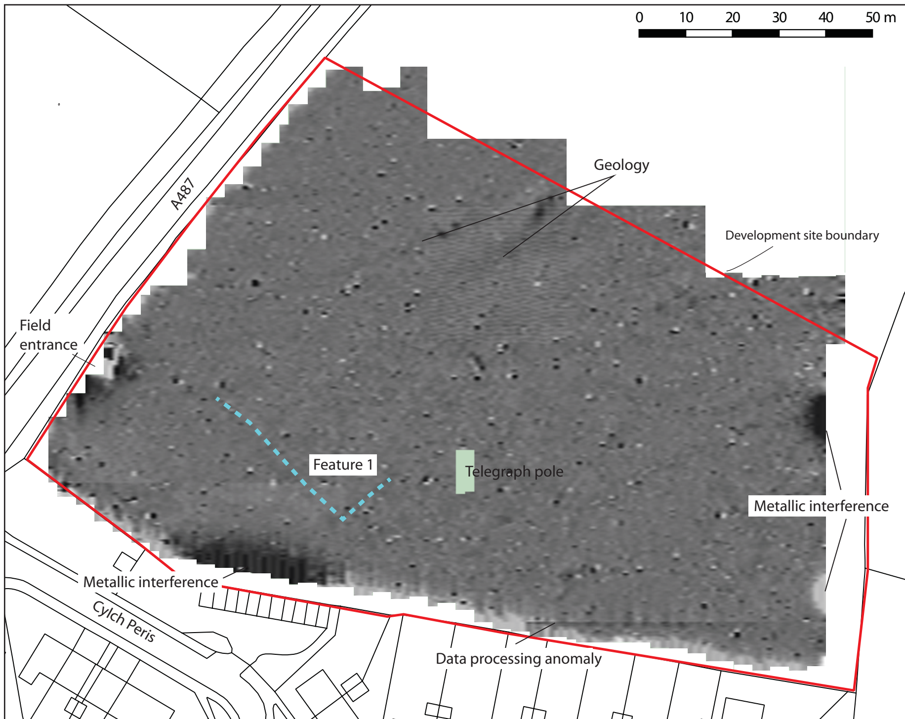
Figure 5: Interpretation layer of geophysical survey results. 1:800 @ A4.
