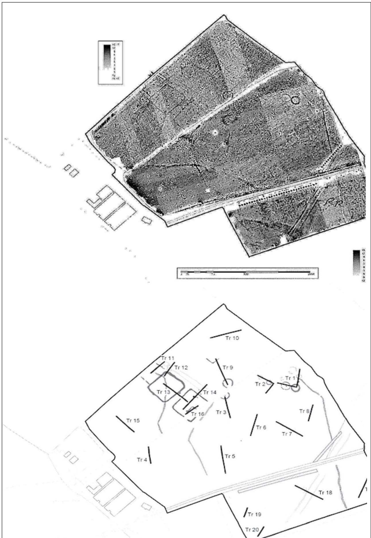
Figure 8 - Geophysical survey results, presented as a grey-scale plot, and original trenches, positioned to target identified geophysical anomalies.
