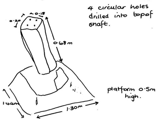
4 circular holes drilled into top of shaft.
