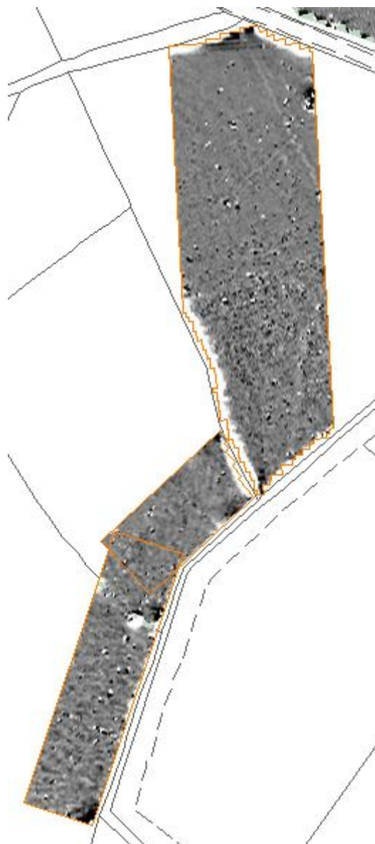
Figure 11: Processed data as grey-scale plot overlaid on local topographical features for the proposed Cable Run area
