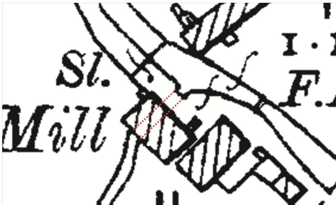
Figure 5: Detail from the 2 nd edition 1:500 scale Ordnance Survey map of 1907, showing the leat entering and exiting within the footprint of the building
