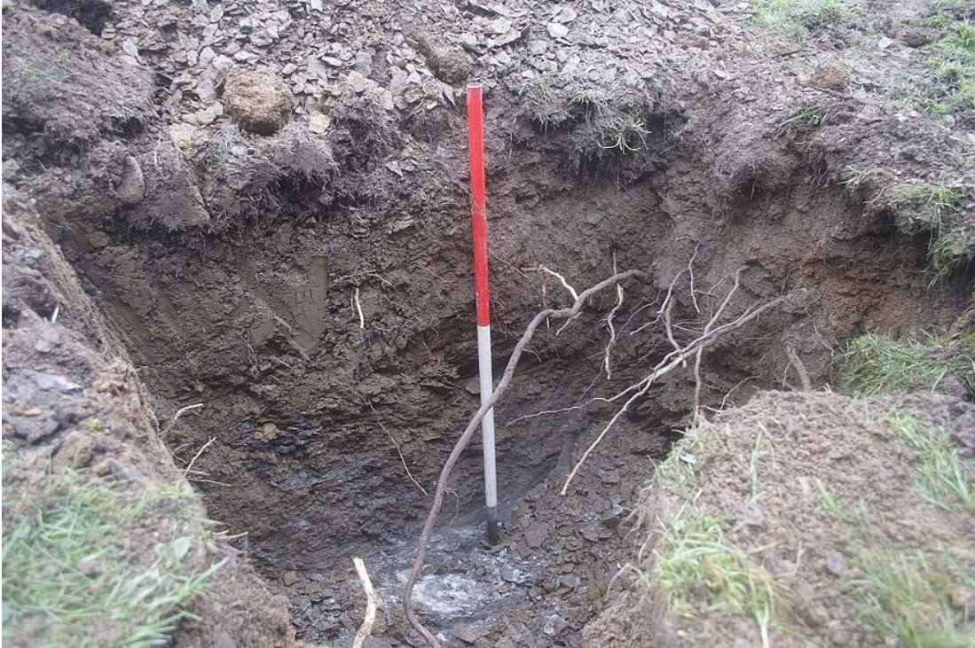
Photo 7: Section of the northernmost soakaway. 1m scale.
