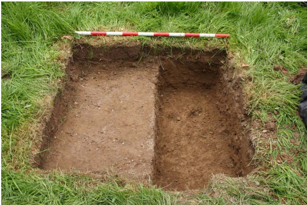
Photo. 42: A test pit illustrating the typical soil profile
