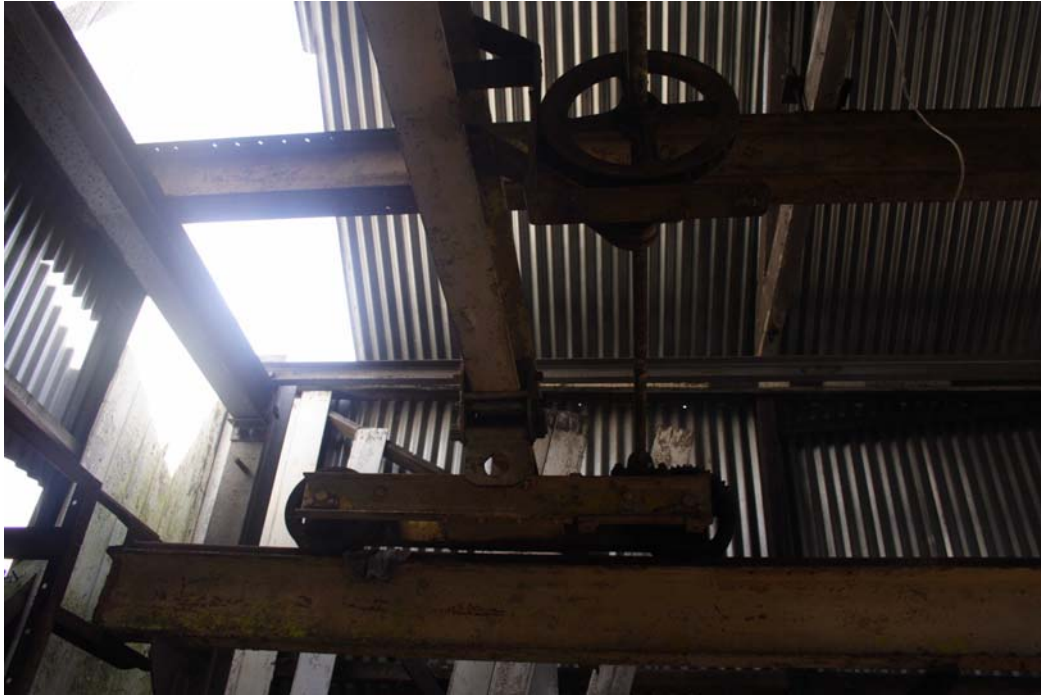
Plate 3977: Metal shed. Later workshop hoist
