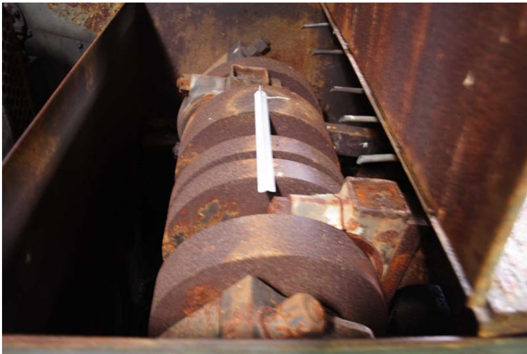
3900: Later pump room. Pump 1 crankshaft
