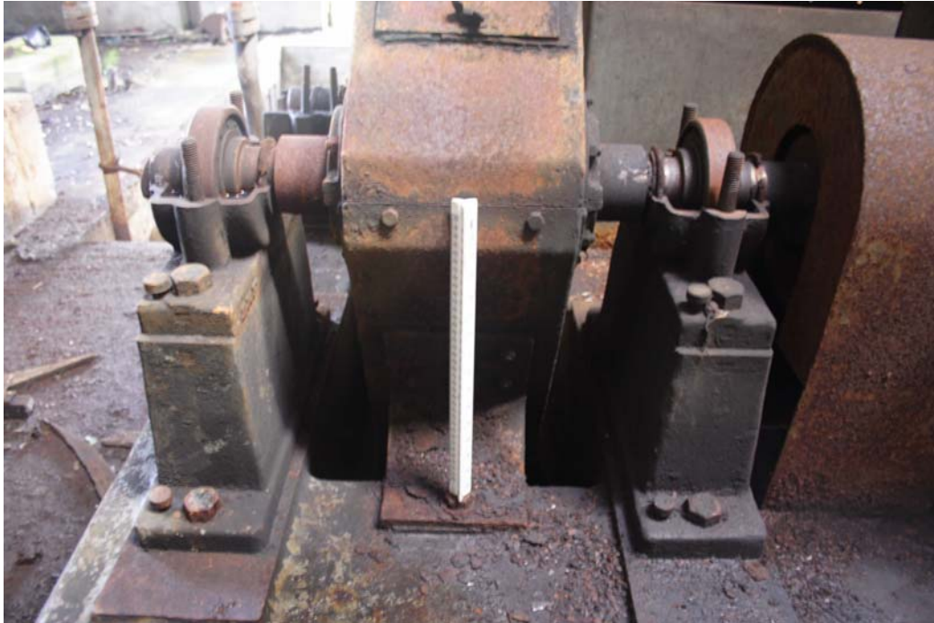
3910: Later pump room. Pump 2 gear wheel and mounting arrangement
