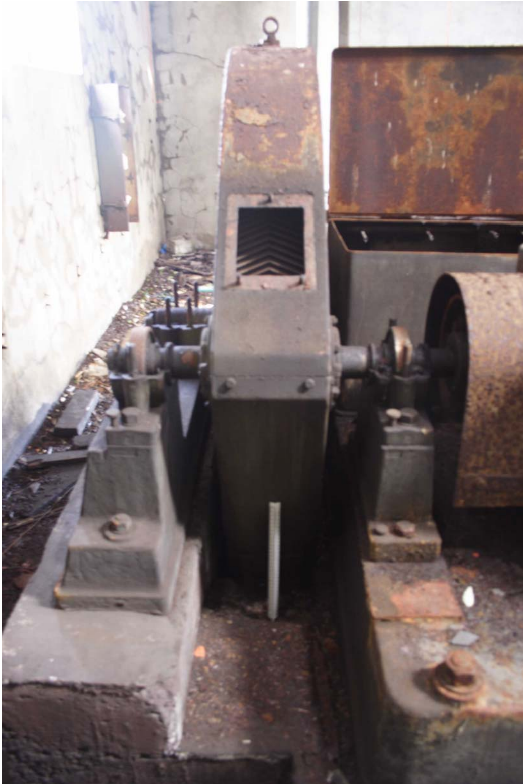
3903: Later pump room. Pump 2 gearwheel set in pit
