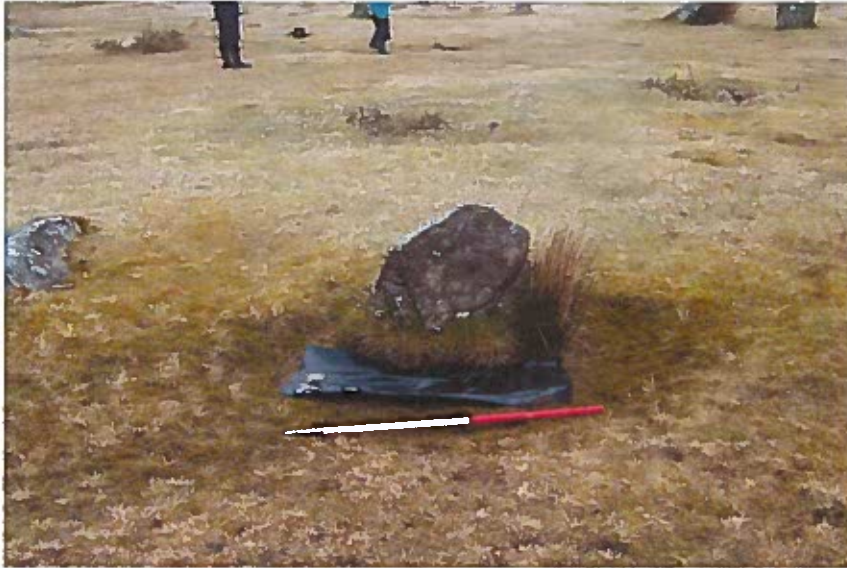
Picture 14 (above) A small piece of Terram in place as a marker, to monitor future erosion problems.
