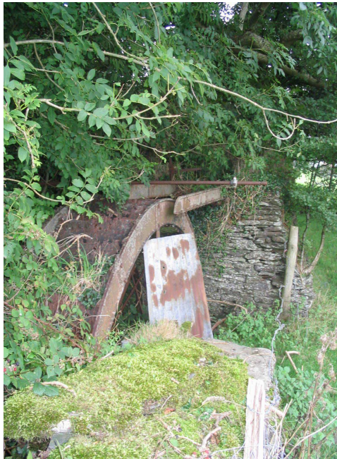
The cast iron water wheel and launder behind Gelynen, once used to power belt driven machinery in the barn nearby.
