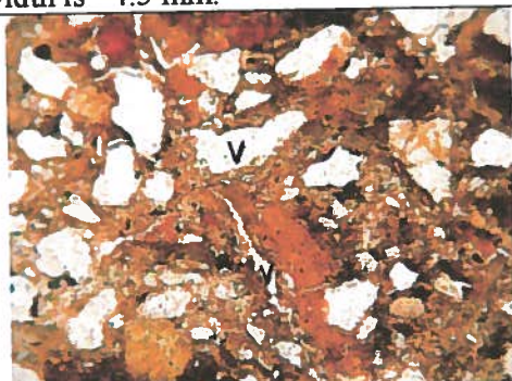
Fig 3: Photomicrograph of M1 showing compact microfabric and voids (V) coated and partially infilled with dusty clay. Plane polarised light (PPL), frame width is ~0.45 mm.
