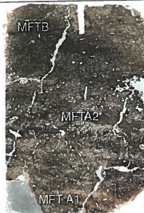
Fig 2: Scan of M6 showing layers – from the bottom upwards: iron-stained MFT A1, MFT A2, and an uppermost humic layer – MFT B. Frame width is ~4.5 mm.
