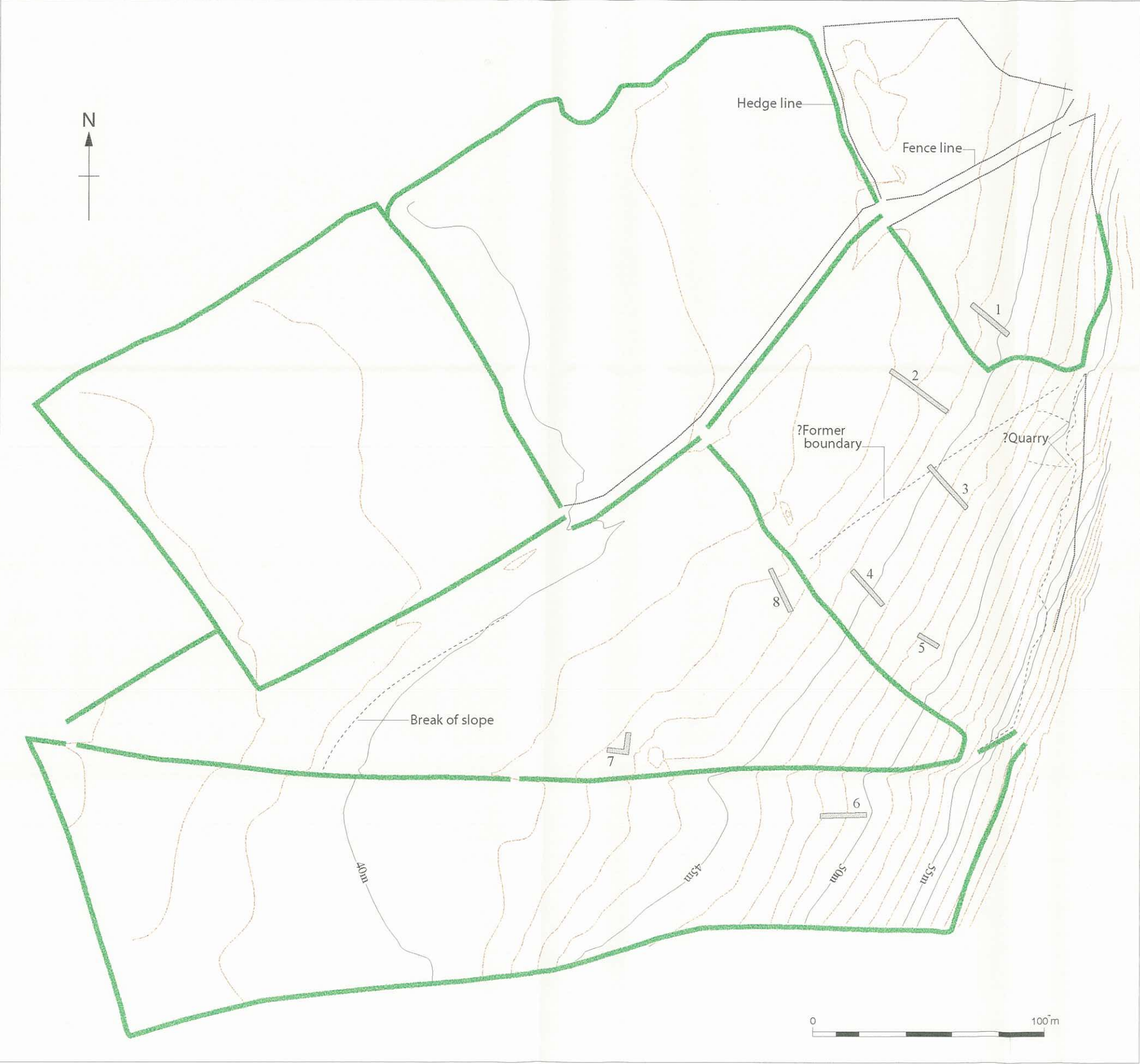
Figure 4: Topographic survey with location of evaluation trenches
