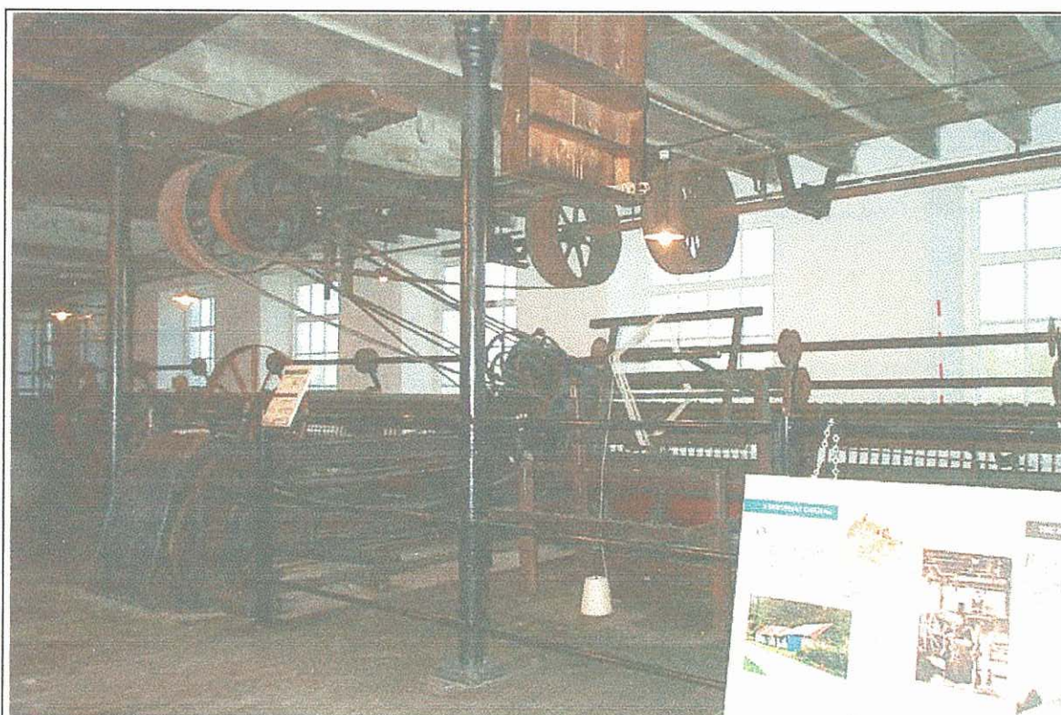
Plate 10: Mill 2, Room K (Gallery 3) showing 1913 mules and belt-drives
