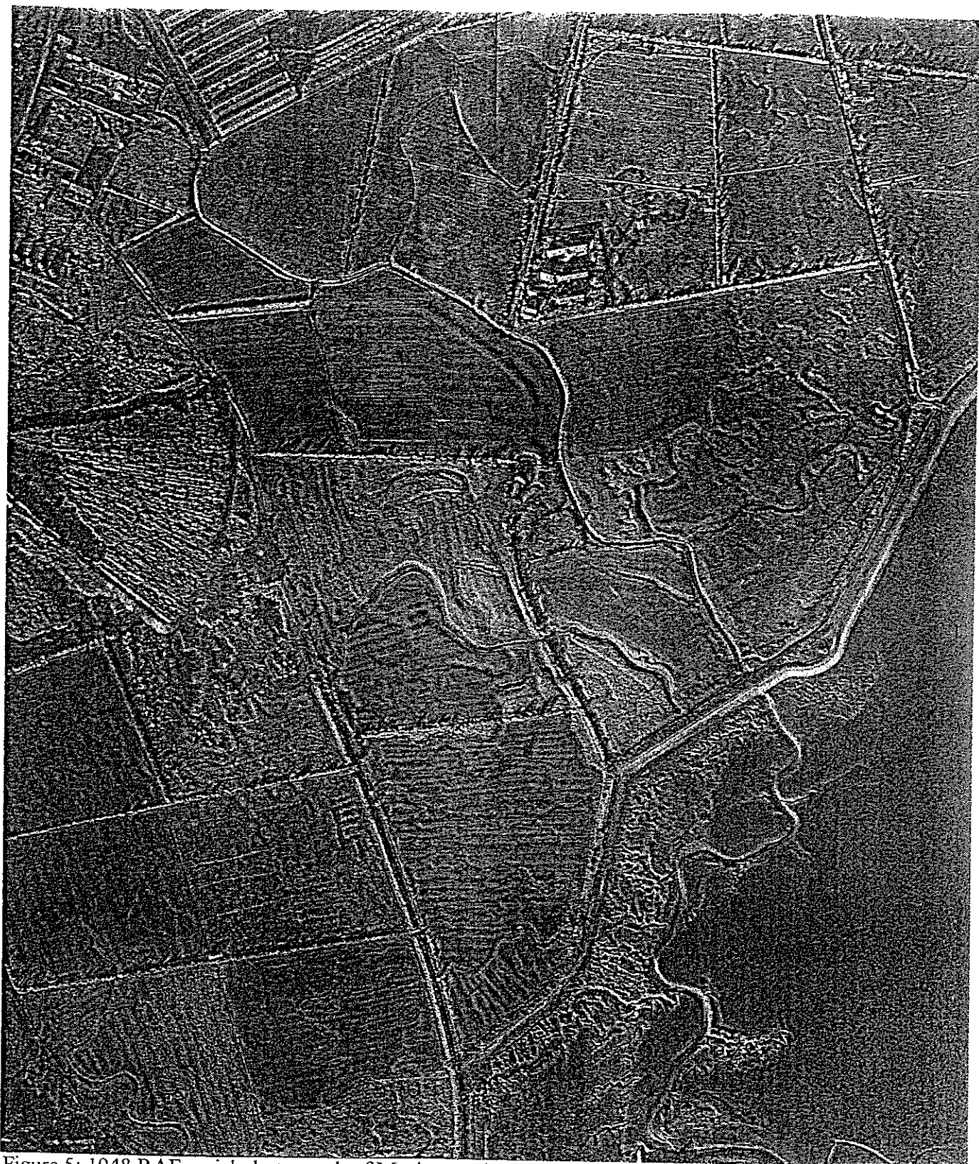
Figure 5: 1948 RAF aerial photograph of Machynys showing the main phases of embankment and the complex pattern of natural and artificial drainage
