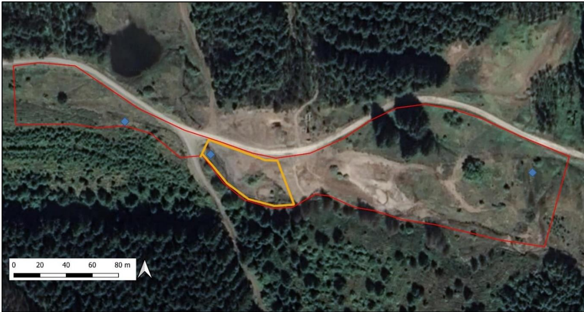
Figure 9: Initial proposed locations for flow monitoring structures (blue) and scour protection works (orange) within the study area. © Google 2024
