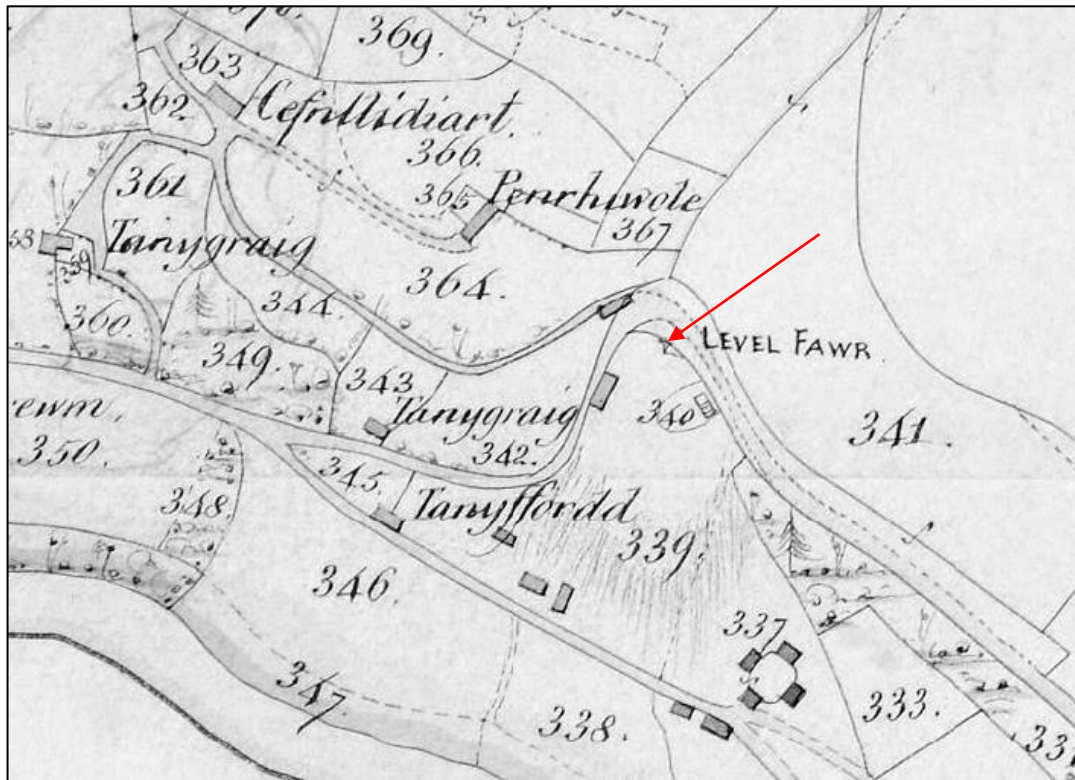
Figure 5: Extract from the 1849 tithe map showing the Level Fawr adit (arrow), with the count house below to the left, and a smithy below to the right. North is to the left.
