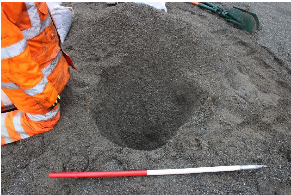
Photograph 13: View north of TP114 during excavation showing mine tailings collapsed into test pit. 1m scale.
