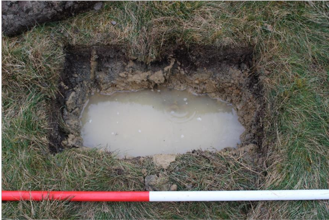
Photograph 8: View north of TP111 that was abandoned due to water ingress. 1m scale
