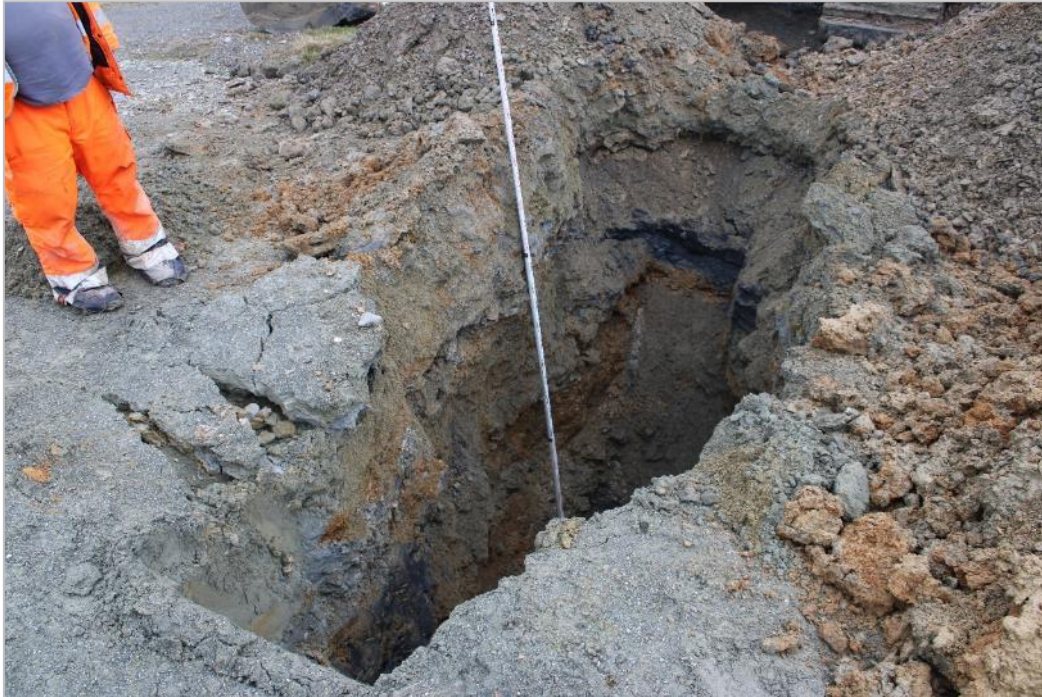
Photograph 11: View west of TP113 fully excavated showing depth of tailings that extended to 3.4m depth, at which point sides of test pit became unstable.
