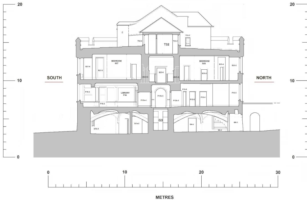
Fig. 178b: Transverse section through Picton Castle east towers, facing west – conjectured medieval
