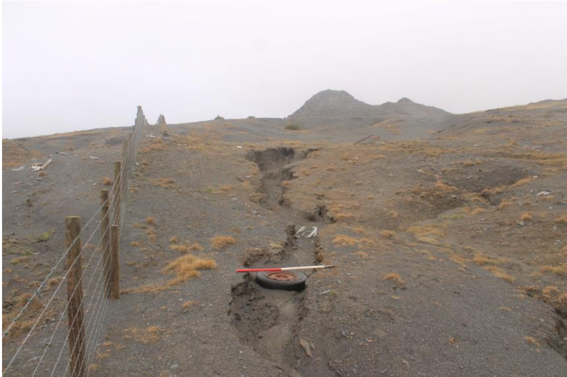
Photo 33: View north along a water channel cutting through spoil tip PRN 97551 . Believed to be one of the main polluting channels, this is the approximate location for a proposed monitoring point. 1m scale.
