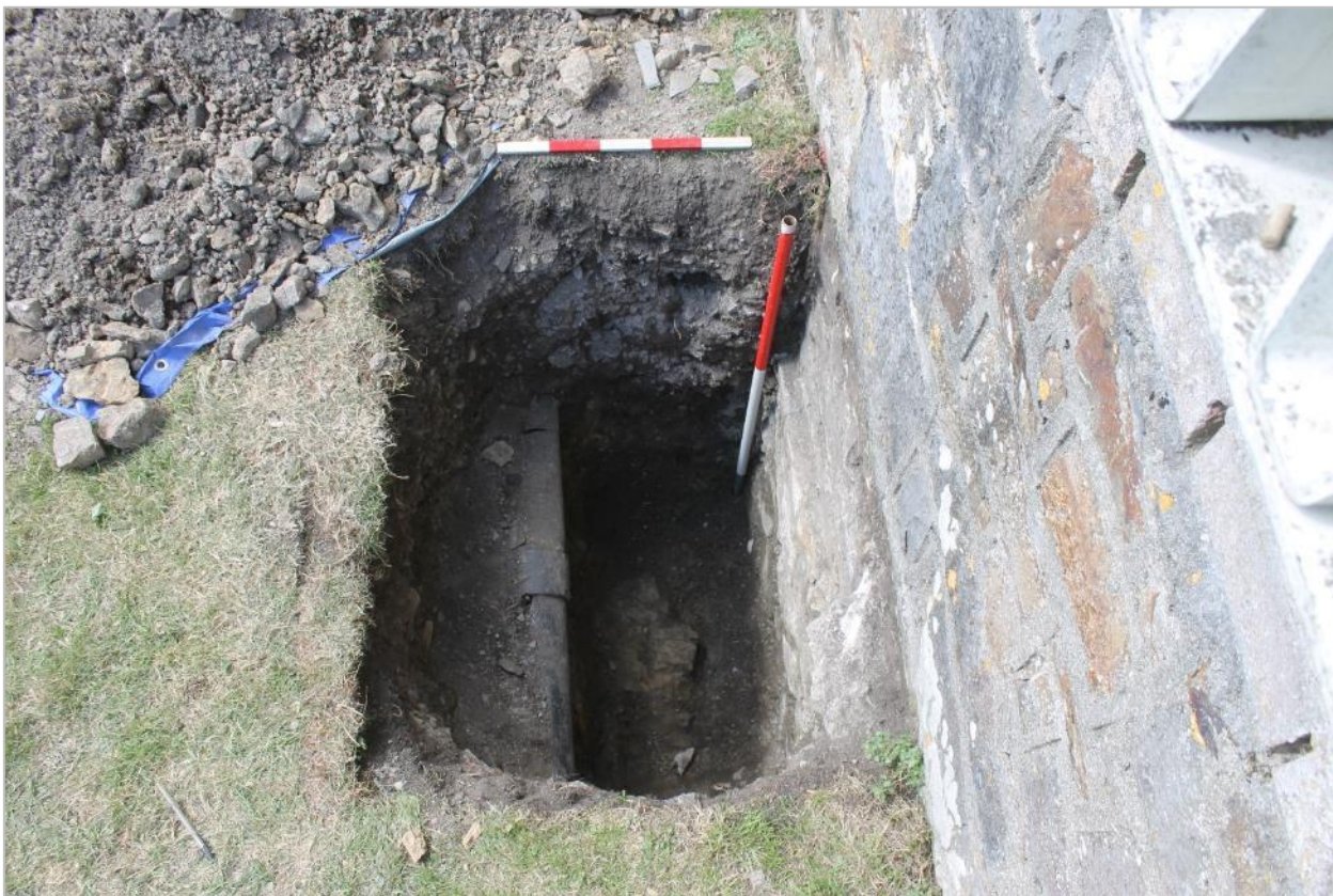
Photo 19: Showing deposits and drainpipe in Test Pit 6. Looking west, 1m & 0.5m scales.
