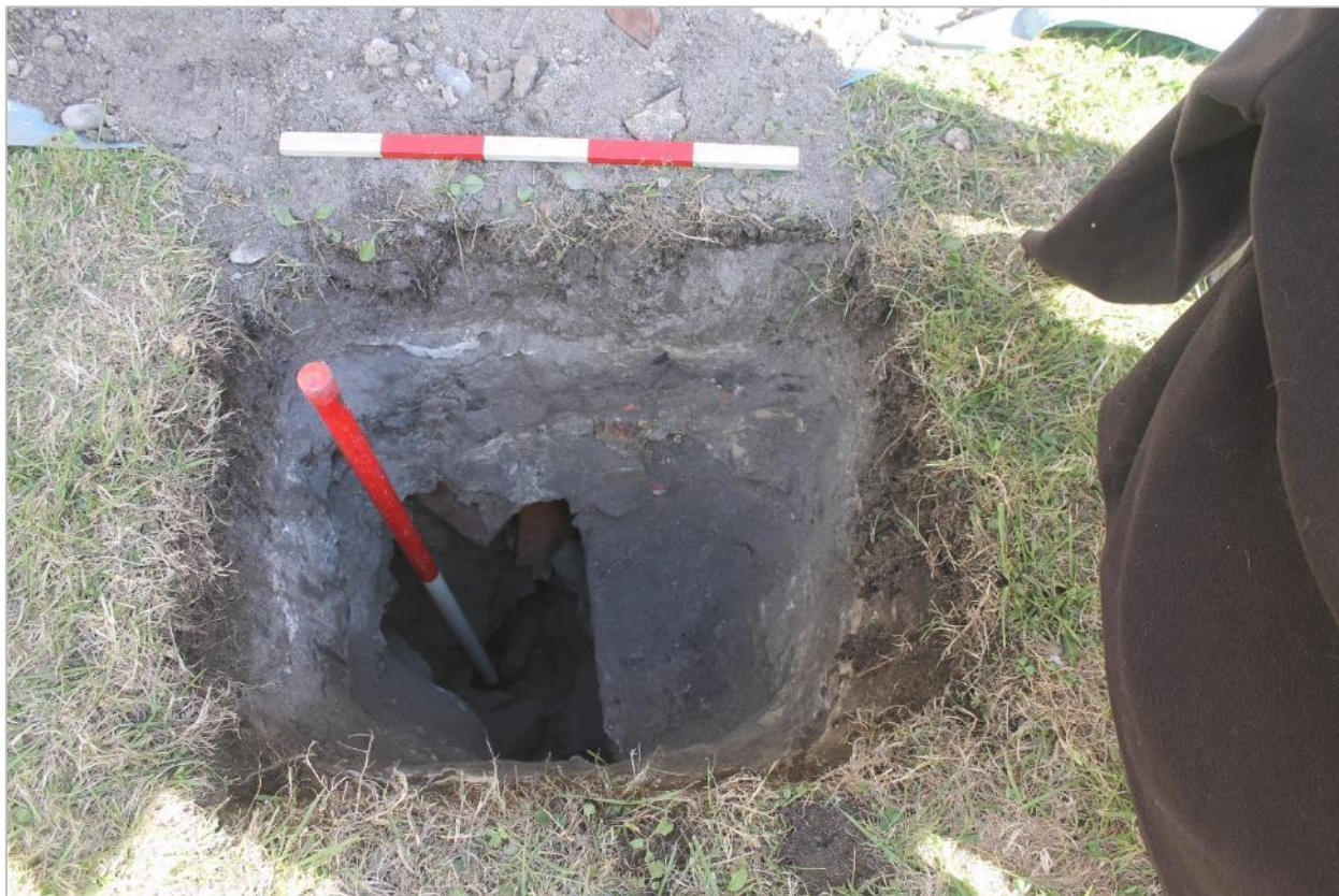
Photo 25: Showing a void revealed below concrete in Test Pit D. Looking north, 0.5m & 1m scales.
