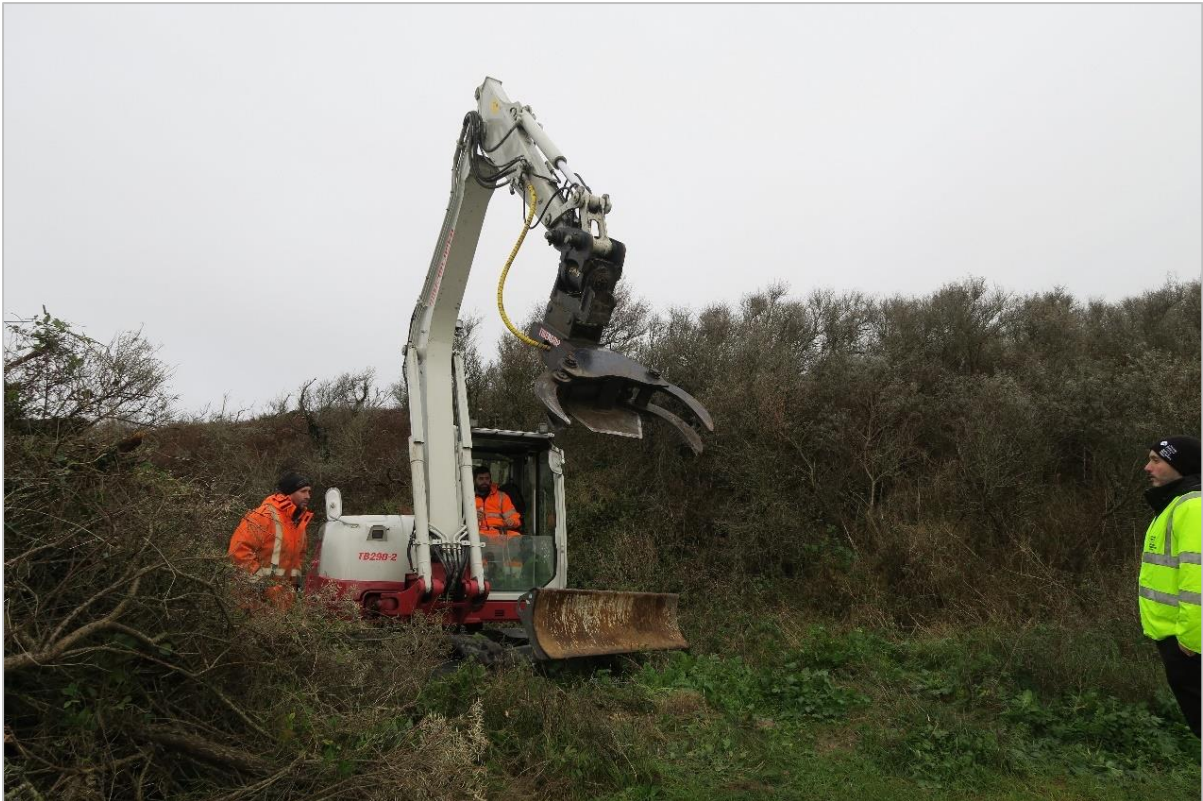
Photo 2: A mechanical excavator equipped with a tree shear attachment (photo by C. Enright, 2021).
