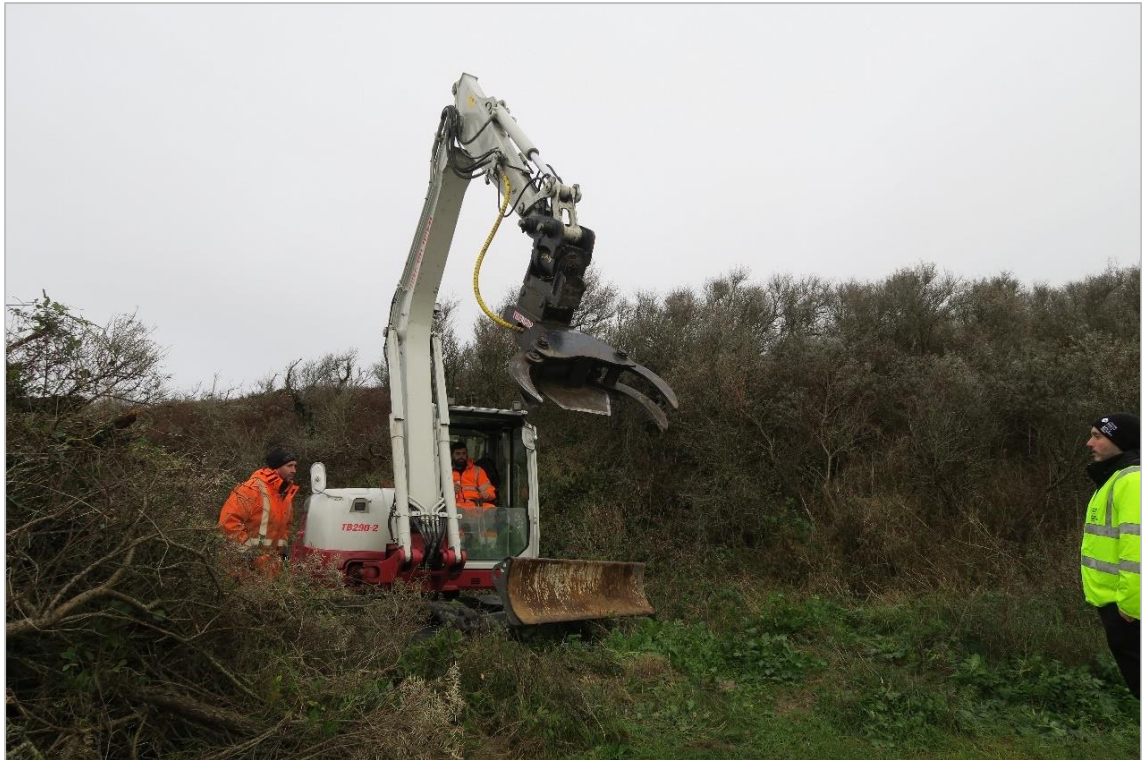
Photo 2: The mechanical excavator is equipped with a tree shear attachment for cutting the buckthorn.
