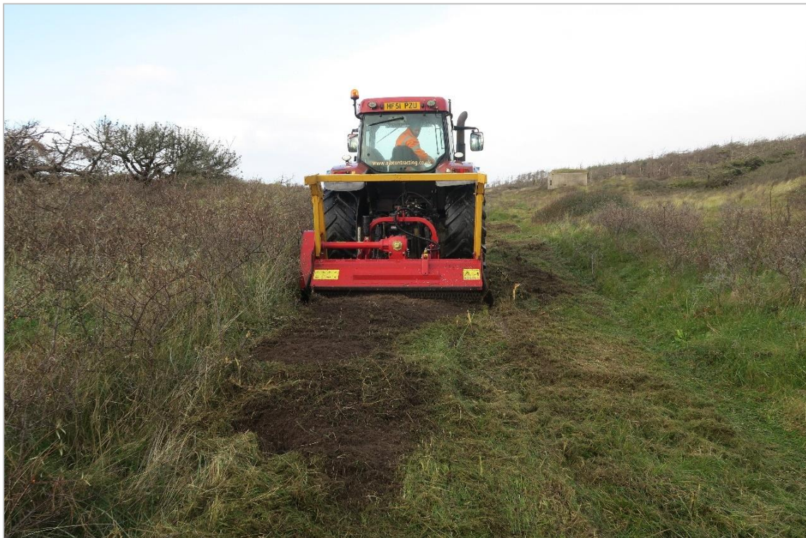
Photo 4: The tracked tractor with a mulching attachment used to clear buckthorn in Area 2.
