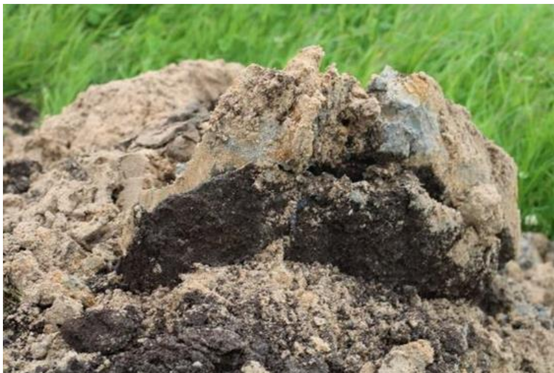
Photograph 4: Showing peaty layers suggesting stabilization within dune layers.
