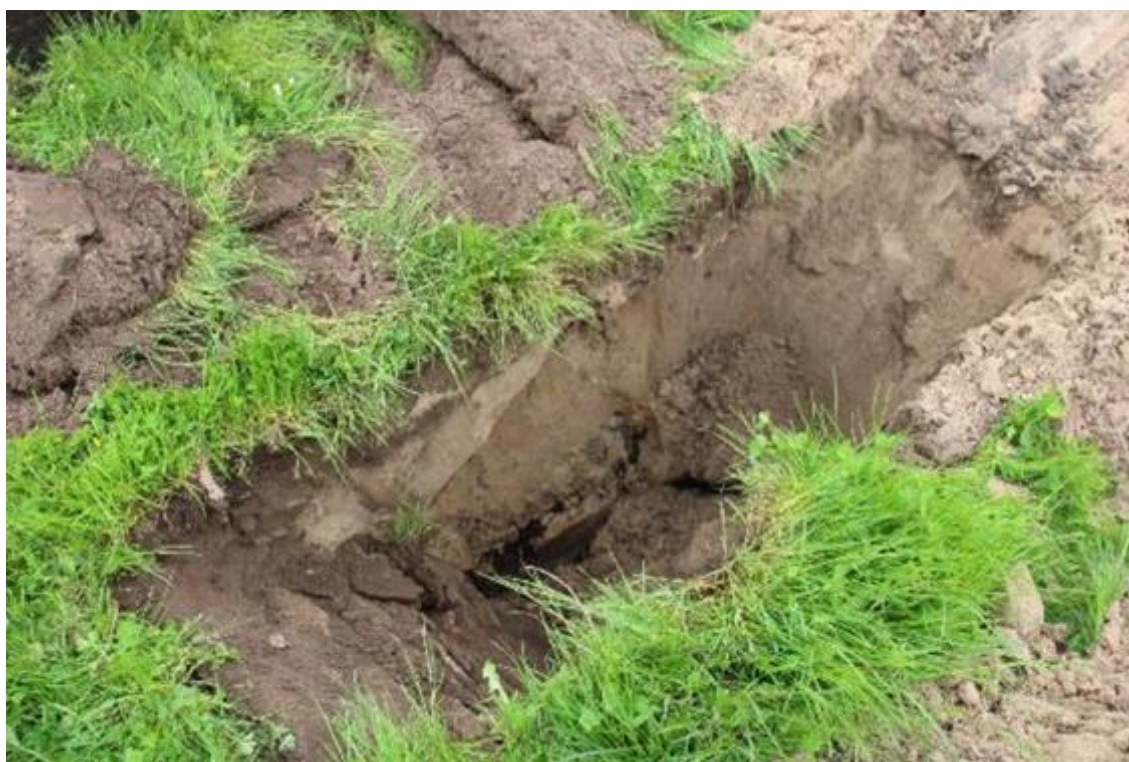
Photograph 3: Showing example of peaty layer in situ approximately 1m beneath ground surface.
