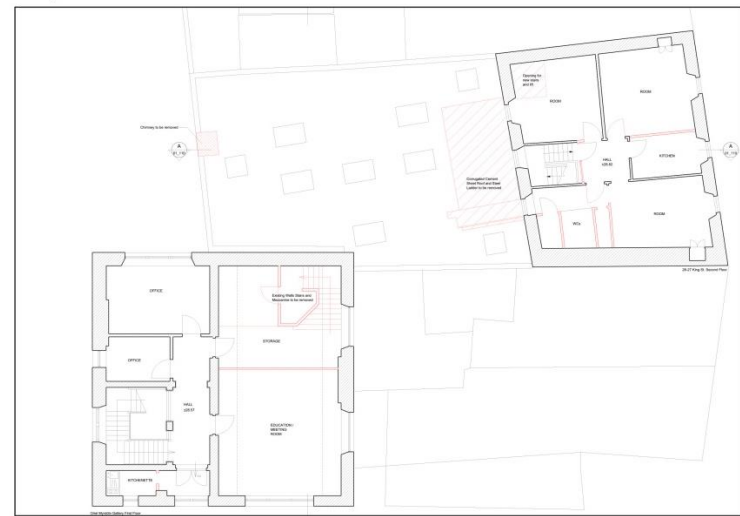
Figure 13: Development proposal plans, showing proposed demolition works to existing structure layouts. Plans taken from the RIBA Stage 3 design report (De Matos Ryan), corresponding to current (June 2021) proposal plans.
