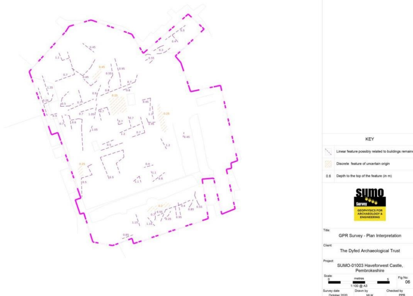
Figure 12: Reproduced figure from the GPR survey (Appendix II - Figure 06), showing interpretation of GPR data. The figure shows the features identified, and the depths at which they were encountered. The full range of GPR survey results, and a full description of the interpreted features, are included in Appendix II.
