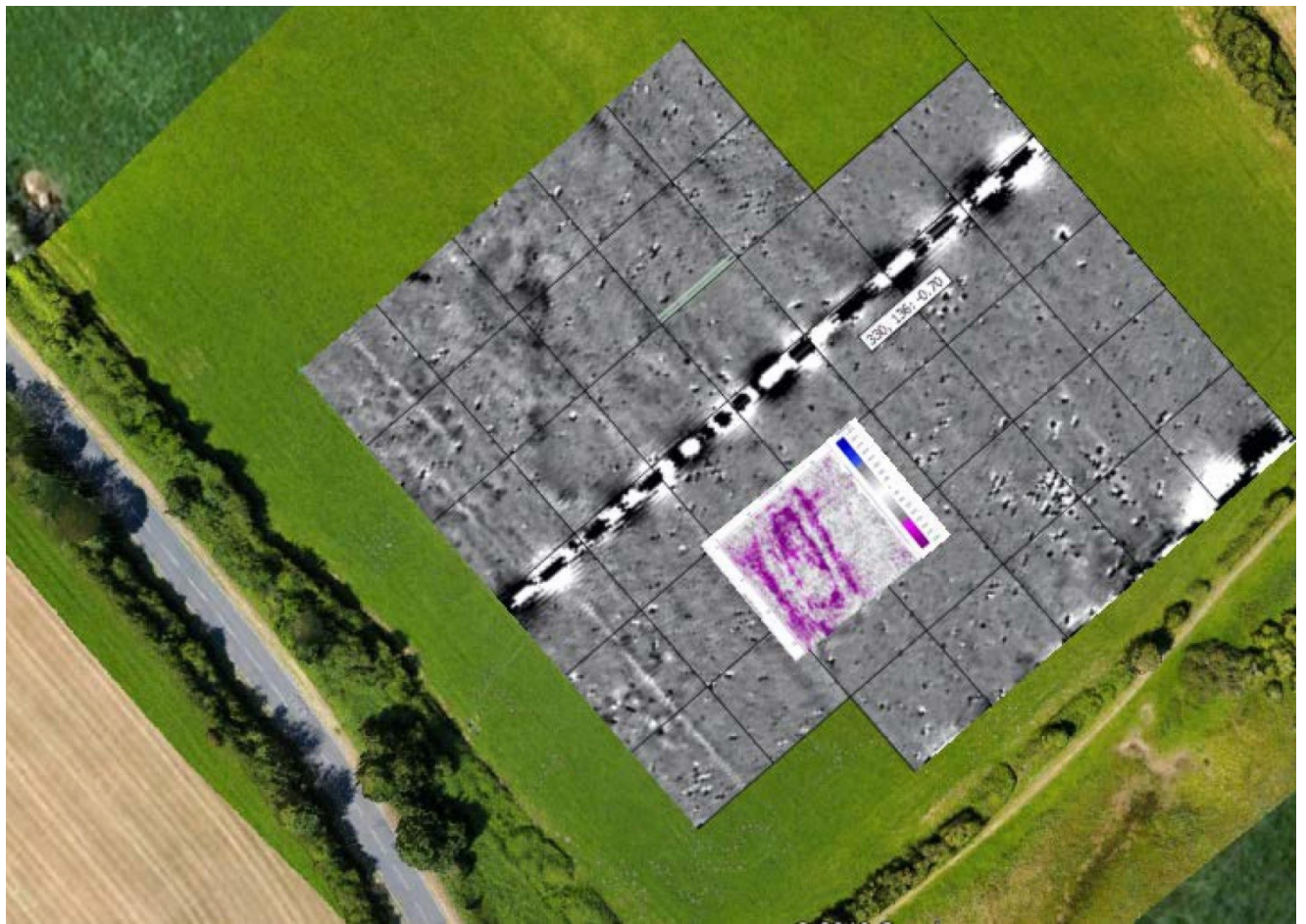
Figure 27: Results of the ground penetrating radar survey that was carried out in the area of the rectangular structure recorded during the geophysical survey (Tim Fletcher, Geoscope).
