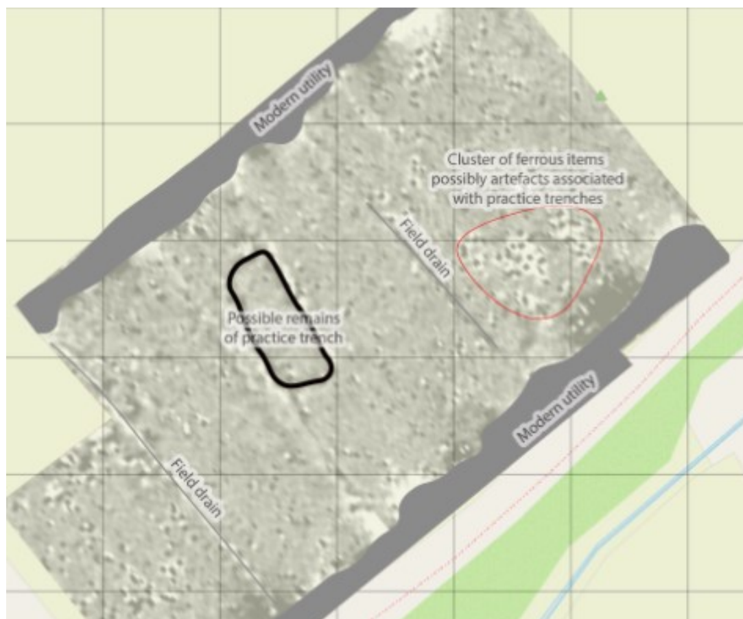
Figure 25: Geophysical survey greyscale results in Area 3 east of the bypass; and interpretation plot below.
