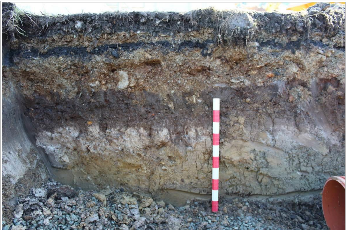
Photo 18: Looking southeast at the detail of the layers of made-up ground at the north end of the trench, with 0.5m scale
