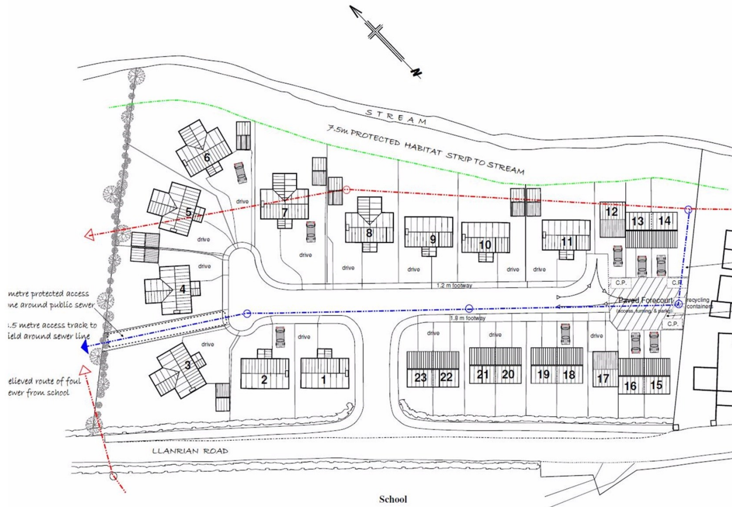
Figure 2: Proposed development layout (plan taken from Pembrokeshire County Council planning website) with line of existing sewer shown in red and proposed realignment in blue.
