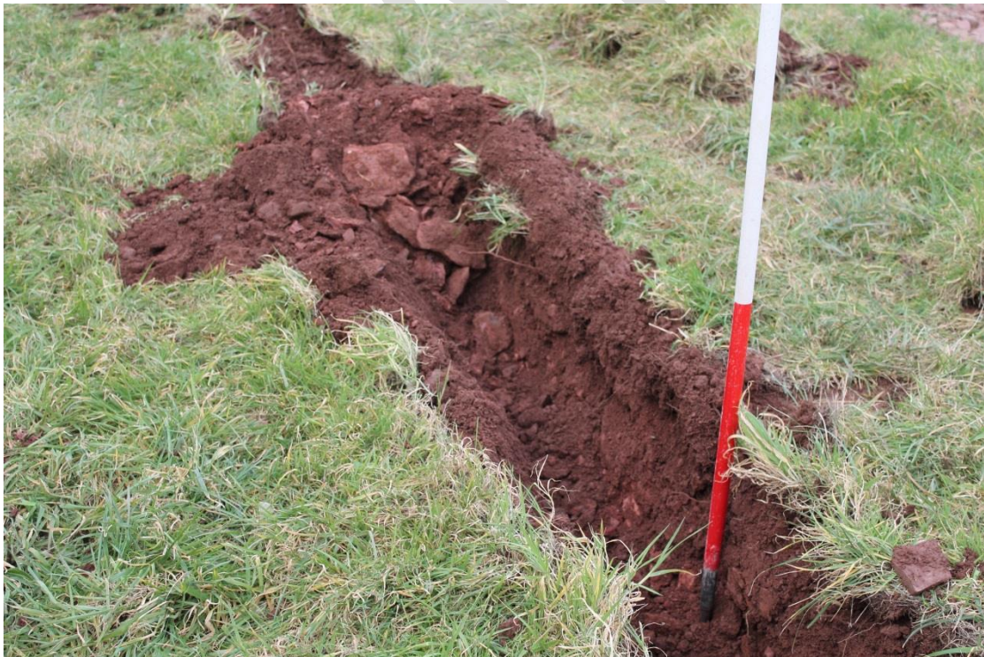
Photo 3: The depth of the bedrock after excavation of the topsoil and subsoil at point B on Figure 11, looking west, with a 1m scale
