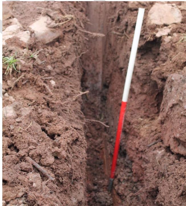
Photo 5: Clay layer above bedrock at point D on Figure 11, looking northeast with a 1m scale
