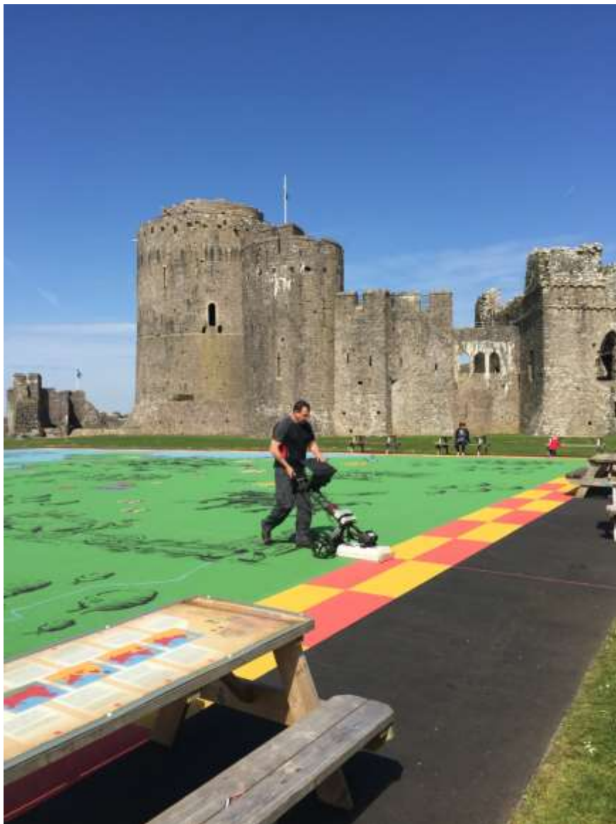
Photo 4: GPR survey being undertaken across the former tennis court area within the outer ward of Pembroke Castle
