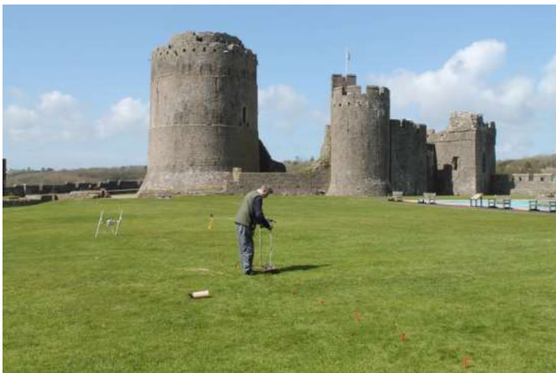
Photo 3: Resistivity survey within the outer ward of Pembroke Castle
