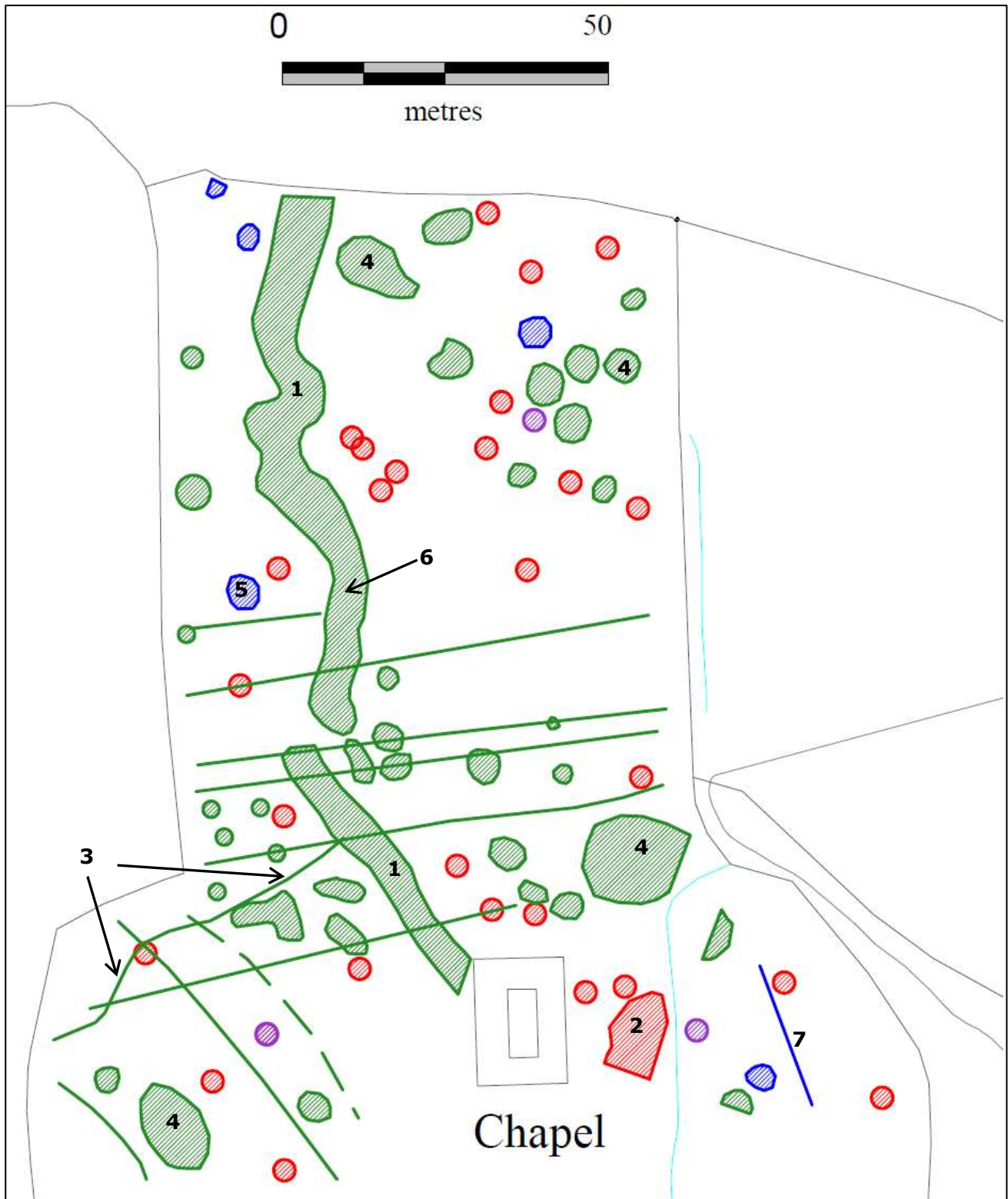
Figure 10: Interpretation plot of survey results, overlaid on local topographical features. (Dipolar features are represented in red; positive features are represented in green; and negative features appear in blue.) Standing stones are also shown, in purple.
