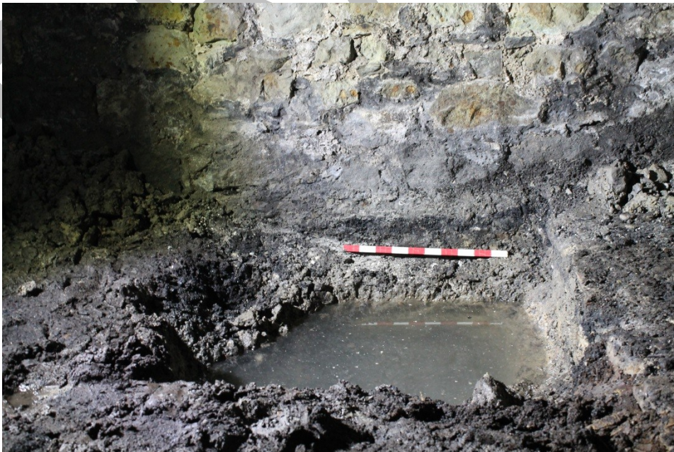
Photo 6: Geotechnical test pit to the base of the south wall in the southwestern corner of the basement. The sub-floor stratigraphy can be seen: Ash and clay layers on top of gravel (under the water). 0.5m scale.
