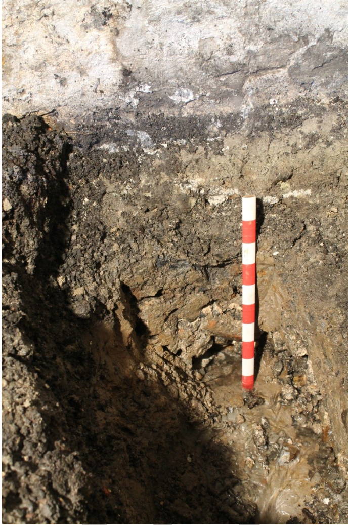
Photo 5: Geotechnical test pit against an internal wall abutting the north wall of the basement. The sub-floor stratigraphy can be seen: Ash and clay layers on top of building rubble and then gravel (water has been pumped out). 0.5m scale.
