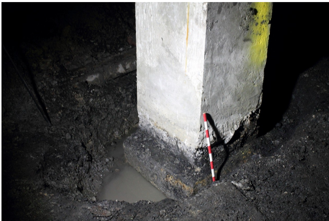
Photo 7: Geotechnical test pit to the base of a pillar in the westernmost room of the basement. Stratigraphy again shows Ash and clay layers on top of gravel (under the water). 0.5m scale.
