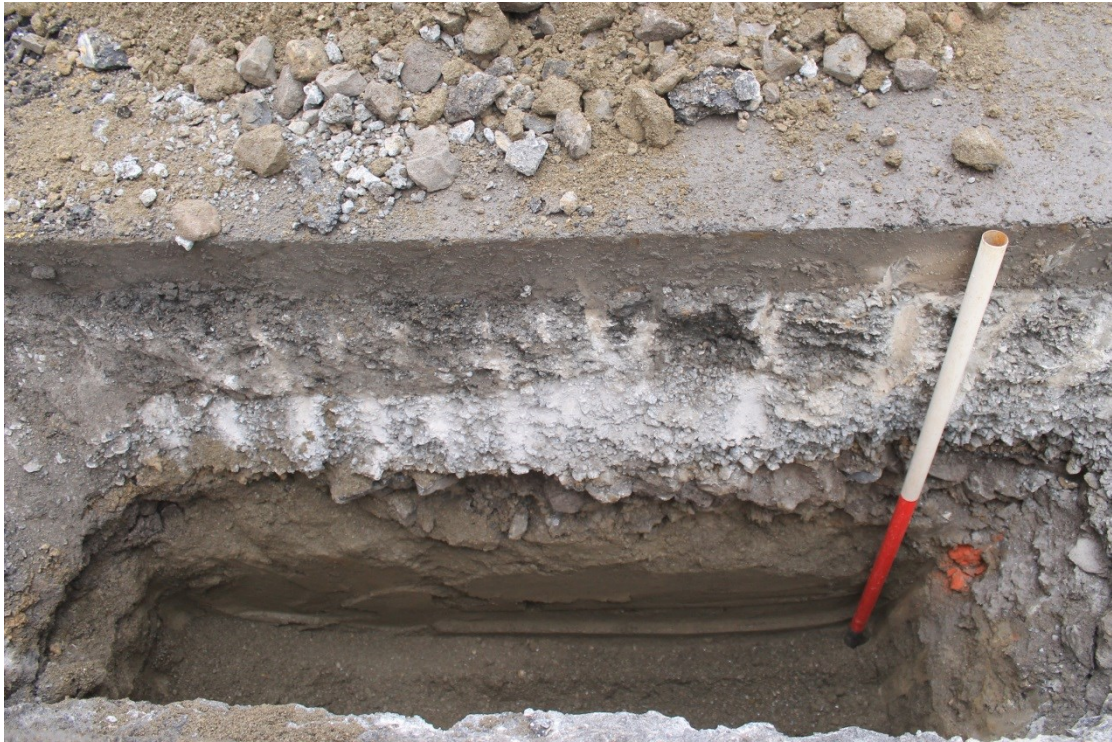
Photo 3: The west face of trial hole T4 showing the natural deposits of sand and gravel that lay directly below the layer of hard core beneath the tarmac. 1m scale
