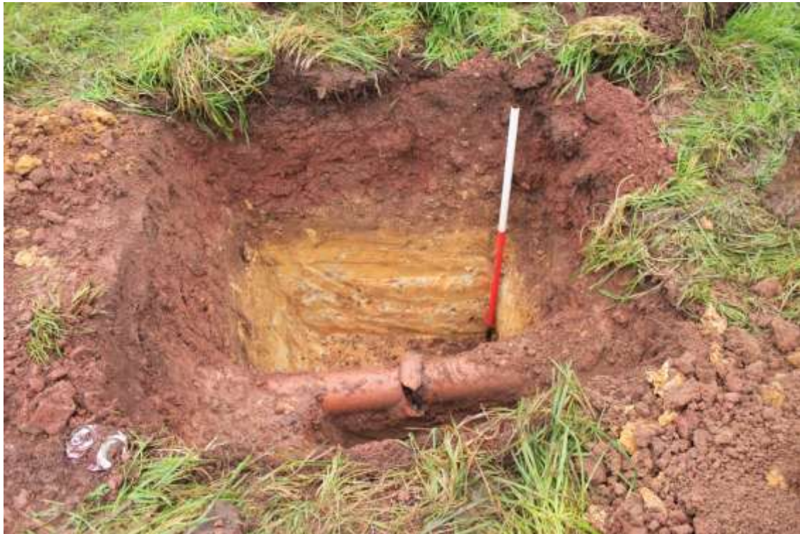
Photo 2: West facing section of TH9 with BT ceramic conduit. 1m scale
