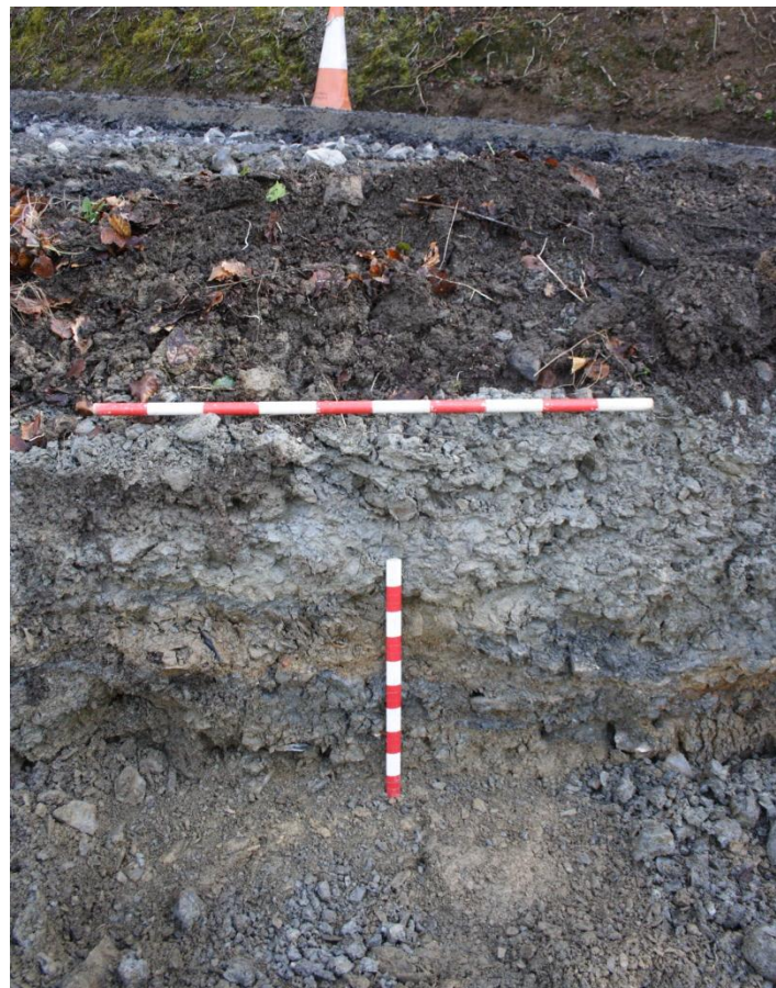
Photo 6: Detail of west facing section through natural bedrock below road make-up layers (material above the 1m horizontal scale bar is re-deposited)
