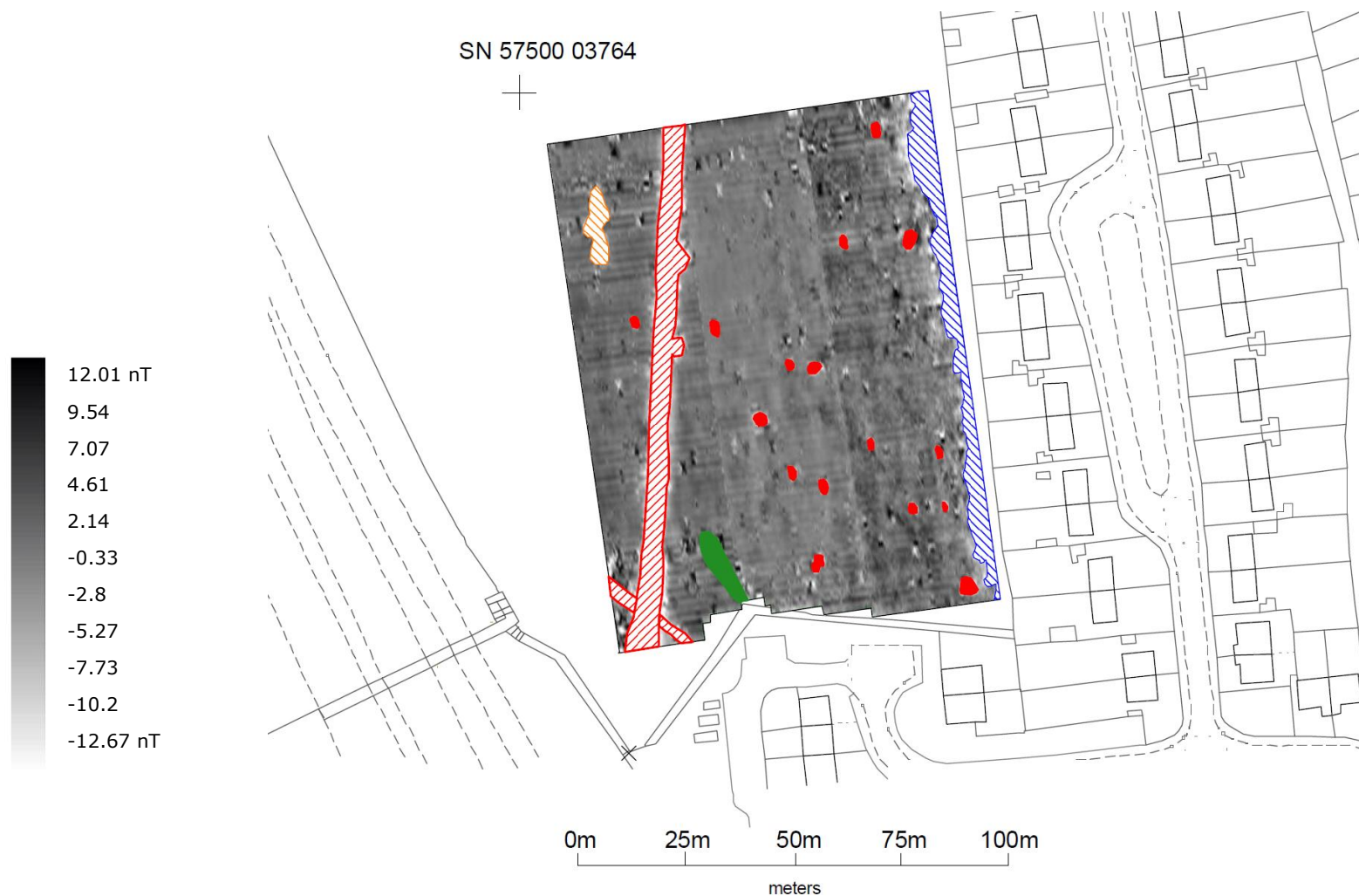
Figure 5: Processed gradiometer survey data – Area 1, greyscale, with interpretation. Red hatchings highlight probable services or ditches, blue and orange hatchings magnetic interference, solid red discrete dipole anomalies and green highlights the main positive anomalies.
