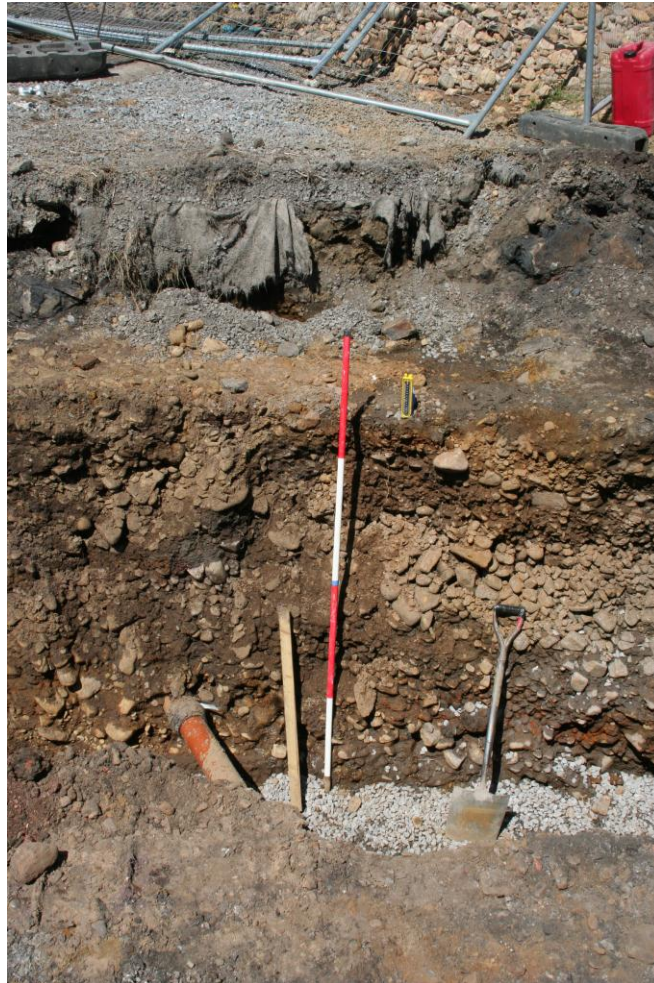
Photo 2: Natural alluvium underlying disturbed upper layers
