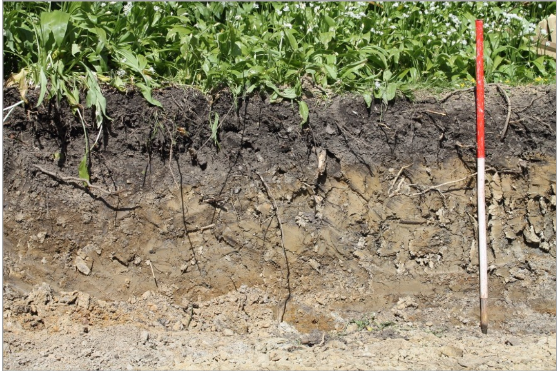
Photo 5: View, looking northwest, of deposits revealed at the northern end of the site. Below the topsoil lies a band of naturally-occurring fluvial clays with the stony subsoil/fragmented bedrock at the base. 1m scale
