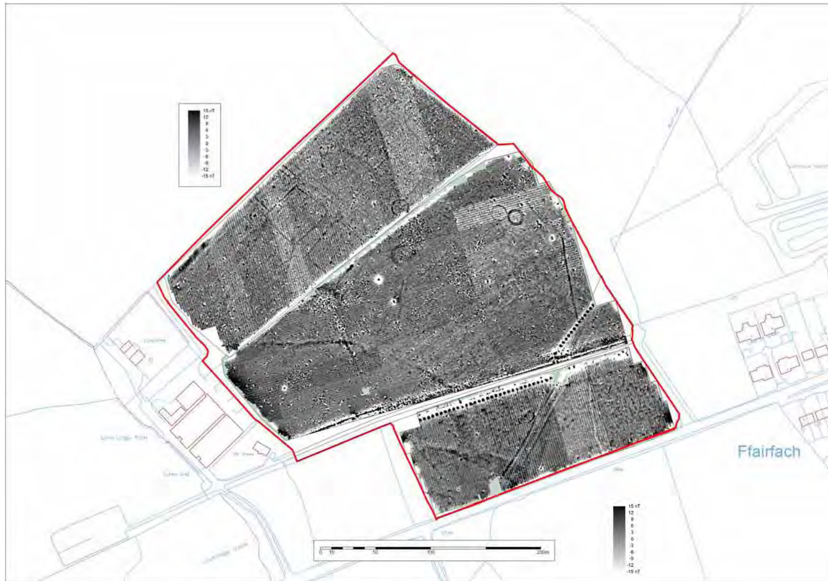
Figure 7: Geophysical survey results, presented as a grey-scale plot, 'clipped' to a range from 10nT to -10nT, and 'despiked'.
