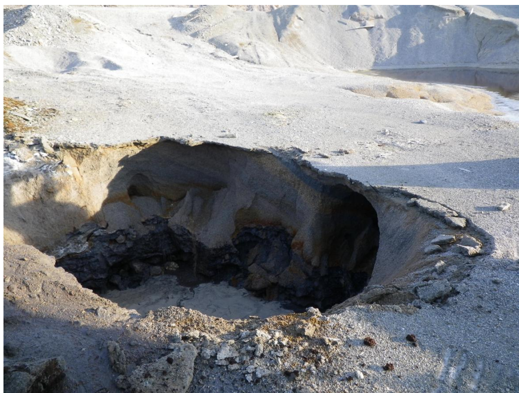
Photo 2: View of Test Pit 1 looking east showing sides subsiding into pit.
