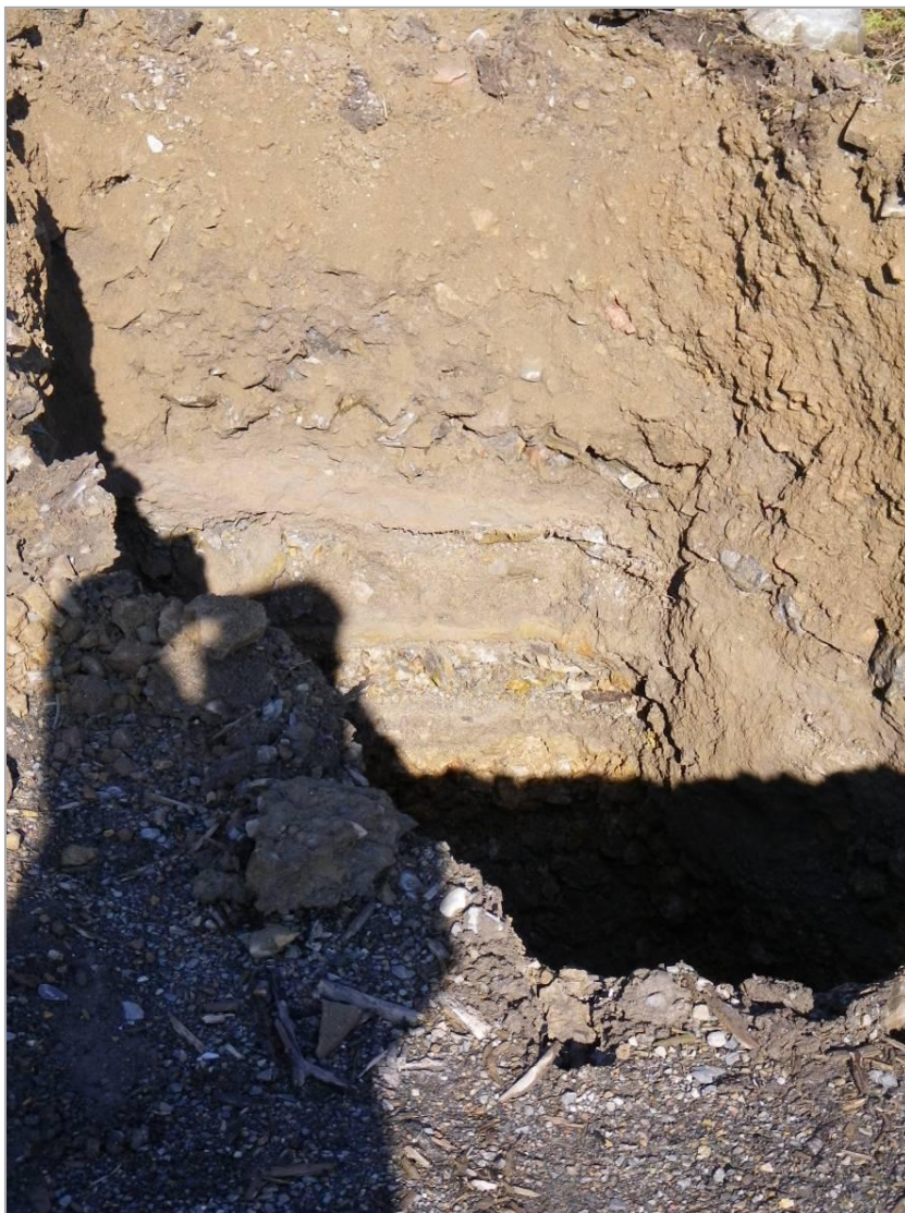
Photo 9 (left): View of Test Pit 3 looking northeast showing detail of layers of compacted tailings interspersed with layers of ore bearing stone.
