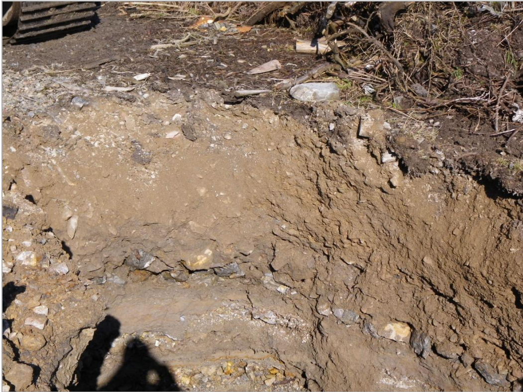
Photo 8: View of Test Pit 3 looking northeast showing detail of layers of compacted tailings interspersed with layers of ore bearing stone.
