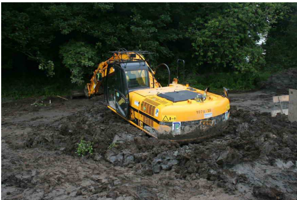
Photo 11: Tracked excavator releasing itself after sinking
