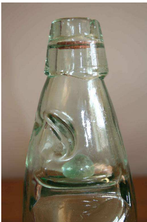
Photo 7: Example of Codd bottle neck showing marble stopper, retaining lugs and rubber washer seal.
